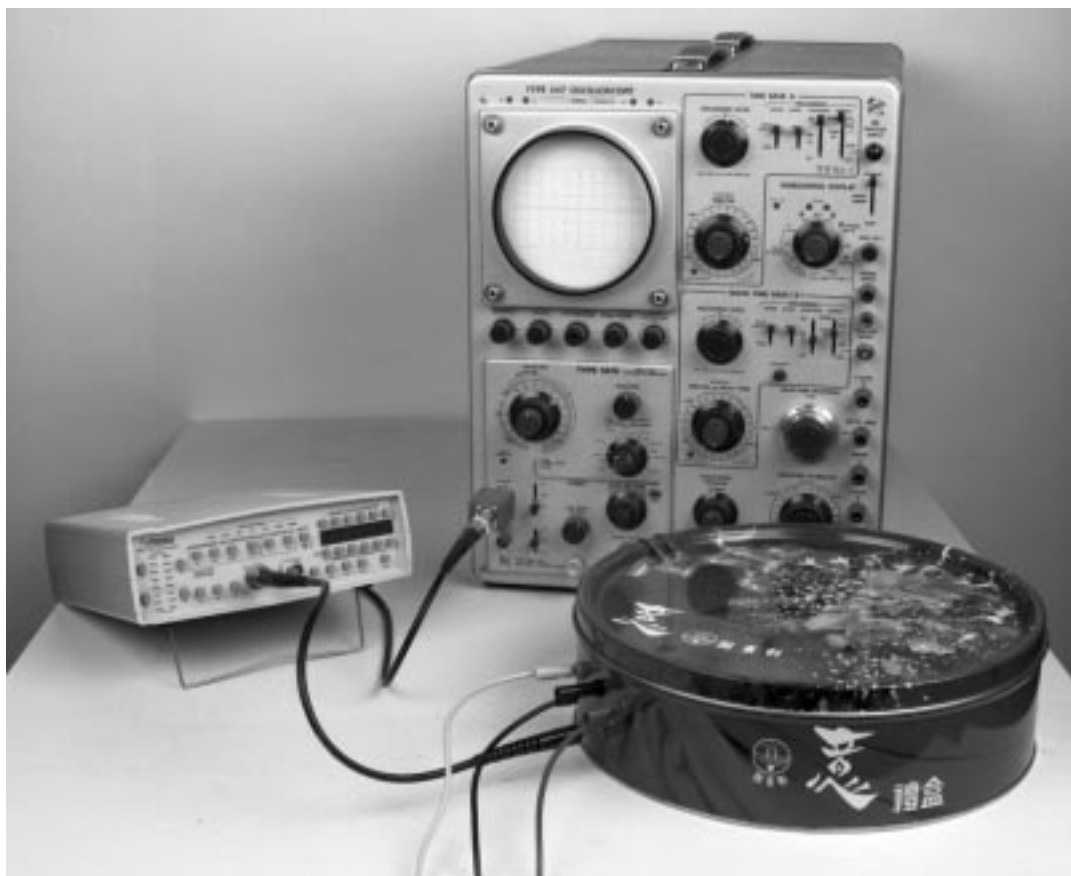
Figure H3. Noise Measurement Test Setup Includes Shielded DAC Breadboard (Foreground), Preamplifier (Left) and Low Pass Filter Attached to Oscilloscope (Center). Measurement Path Is Fully Coaxial
