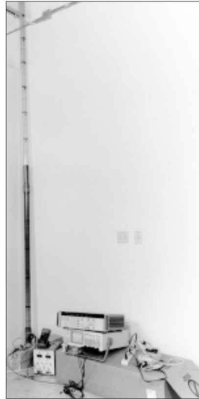
Figure 150. Test Setup for Water-Column Sensor
