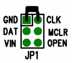
Figure 1. Jumper selection to suspend µcontroller operation
