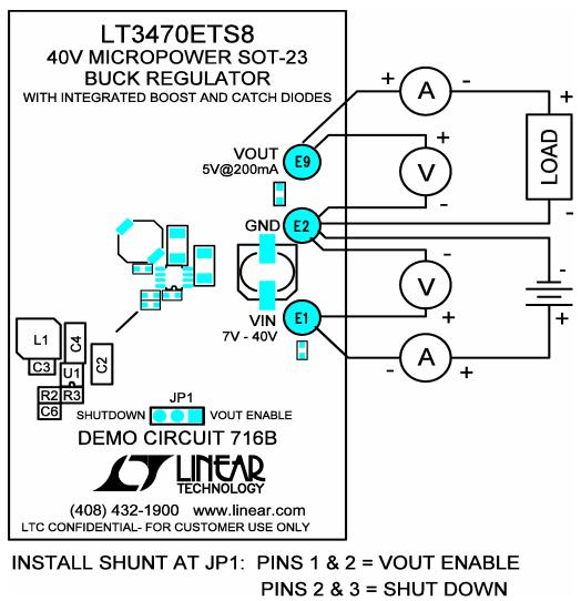
Figure 1. Proper Measurment Equipment Setup
