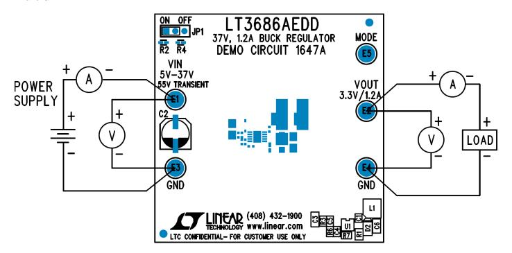
Figure 1. Proper Measurement Equipment Setup
