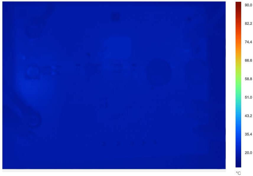
Figure 15. DC2814A-C Thermal Performance at 45V IN (Pass-Thru), 45V OUT , 2A Load Current
