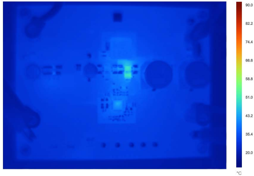
Figure 9. DC2814A-C Thermal Performance at 28V IN (Boost), 36V OUT , 2A Load Current
