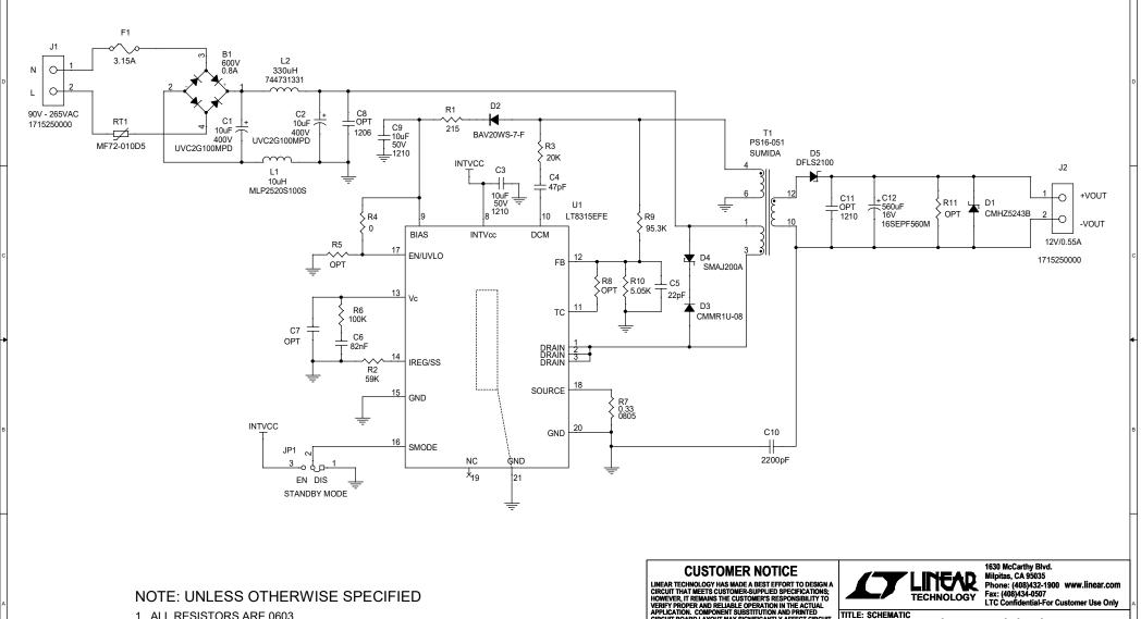
1. ALL RESISTORS ARE 0603. ALL CAPACITORS ARE 0603. LINEAR TECHNOLOGY HAS MADE A BEST EFFORT TO DESIGN A CIRCUIT THAT MEETS CUSTOMER SUPPLIED SPECIFICATIONS: HOWEVER, IT REMAINS THE CUSTOMER'S RESPONSIBILITY OF VERIFY PROPER AND RELIABLE OPERATION IN THE ACTUAL APPLICATION. COMPONENT SUBSTITUTION AND PRINTED CIRCUIT BOARD LAYOUT MAY SIGNIFICANTLY AFFECT CIRCUIT PEPFORMANCE OR RELIABILITY. CONTACT LIMEAR TECHNOLOGY APPLICATIONS ENGINEERING FOR ASSISTANCE.
