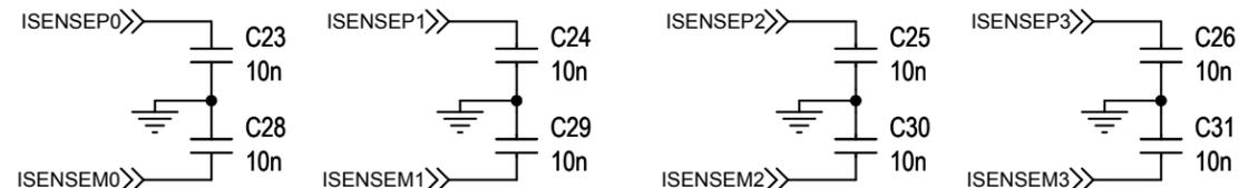
INPUT FILTERS FOR CURRENT SENSING PLACE CLOSE TO LTC2974
