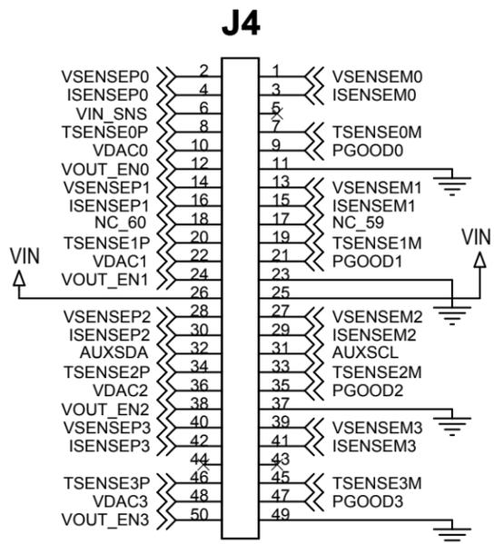
BOARD TO BOARD CONNECTOR MATES WITH DC1810A
