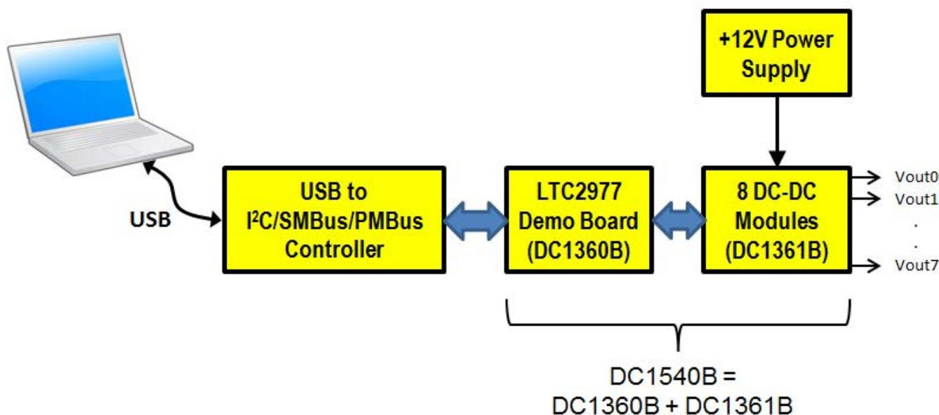
Figure 1. Single LTC2977 Demo Setup Using DC1540B
