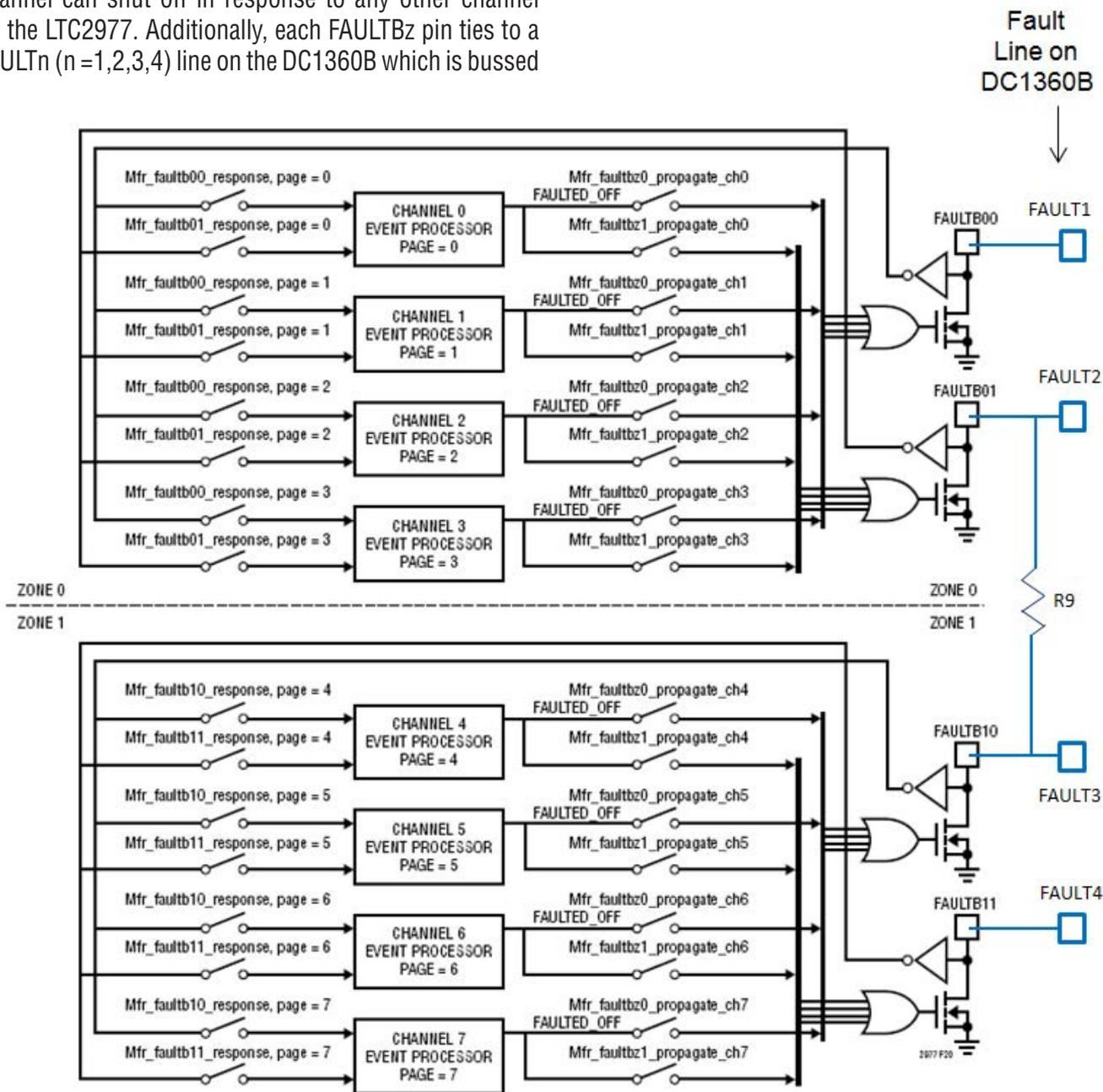
Figure 13. Fault Zones and Fault Pins on DC1360B
