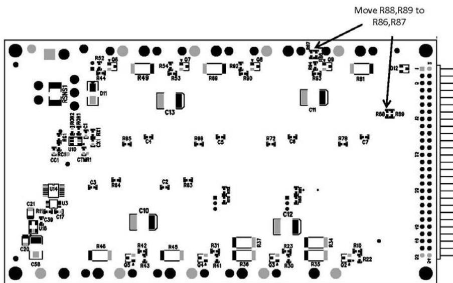
Figure 11. Current Sensing Modifications (Bottom Side of Board)
