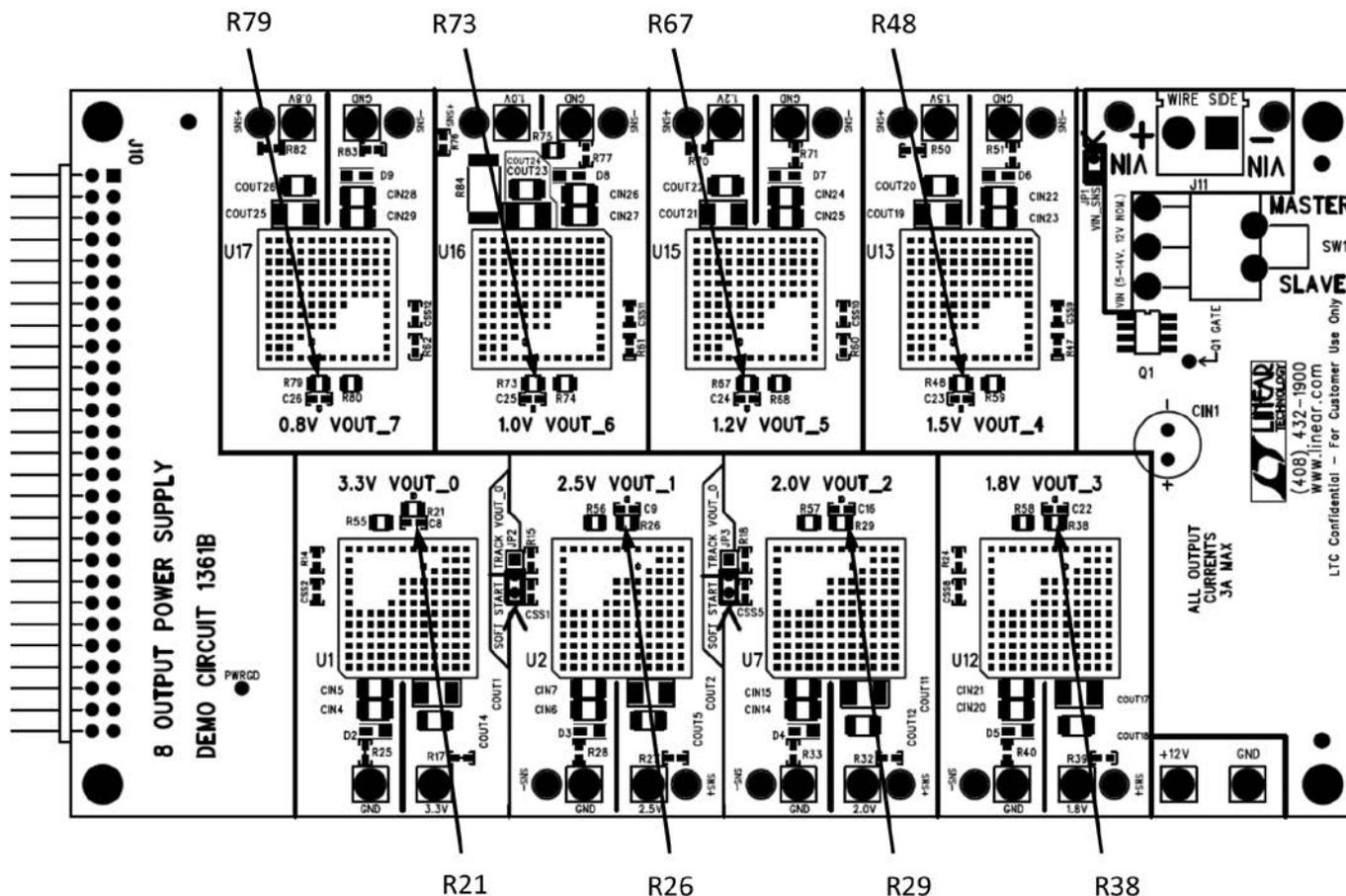
Figure 9. DC1361B Output Voltage Setting Resistor Locations
