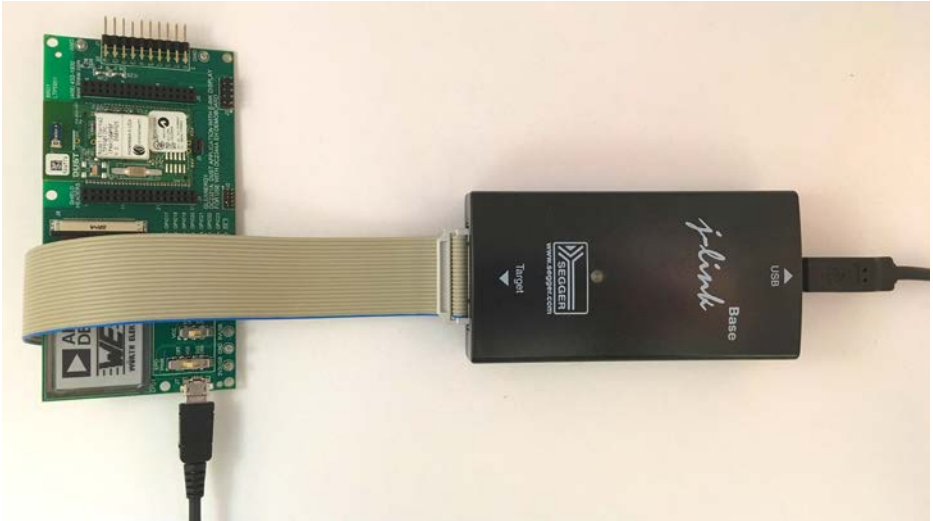
Figure 9b. JTAG Connection with Standard Connector (Not Populated, See BOM)
