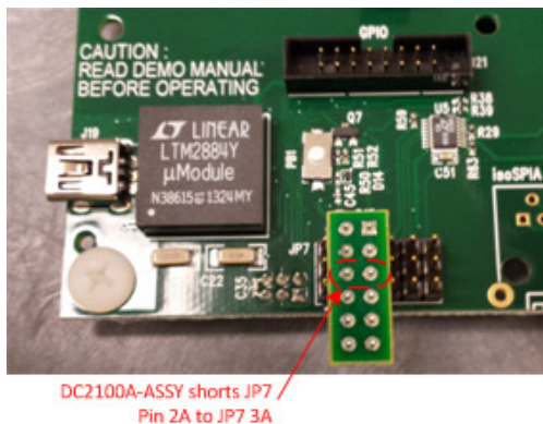
Figure 15 - JP7 Placement to Force Bootloader Mode
