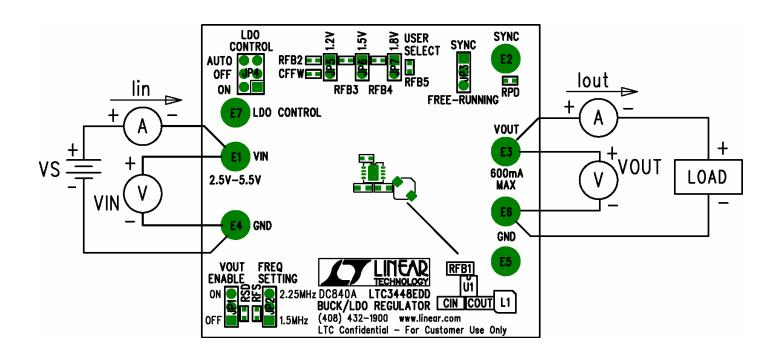
Figure 1. Proper Measurement Equipment Setup
