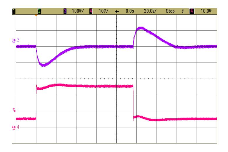
Figure 3. Load Step Response
