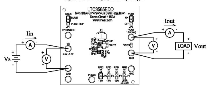
Figure 2. Proper Measurement Equipment Setup
