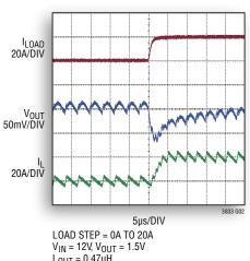
$L_{OUT} = 0.47 \mu H,$  $C_{OUT} = 660 \mu F + 200 \mu F$
