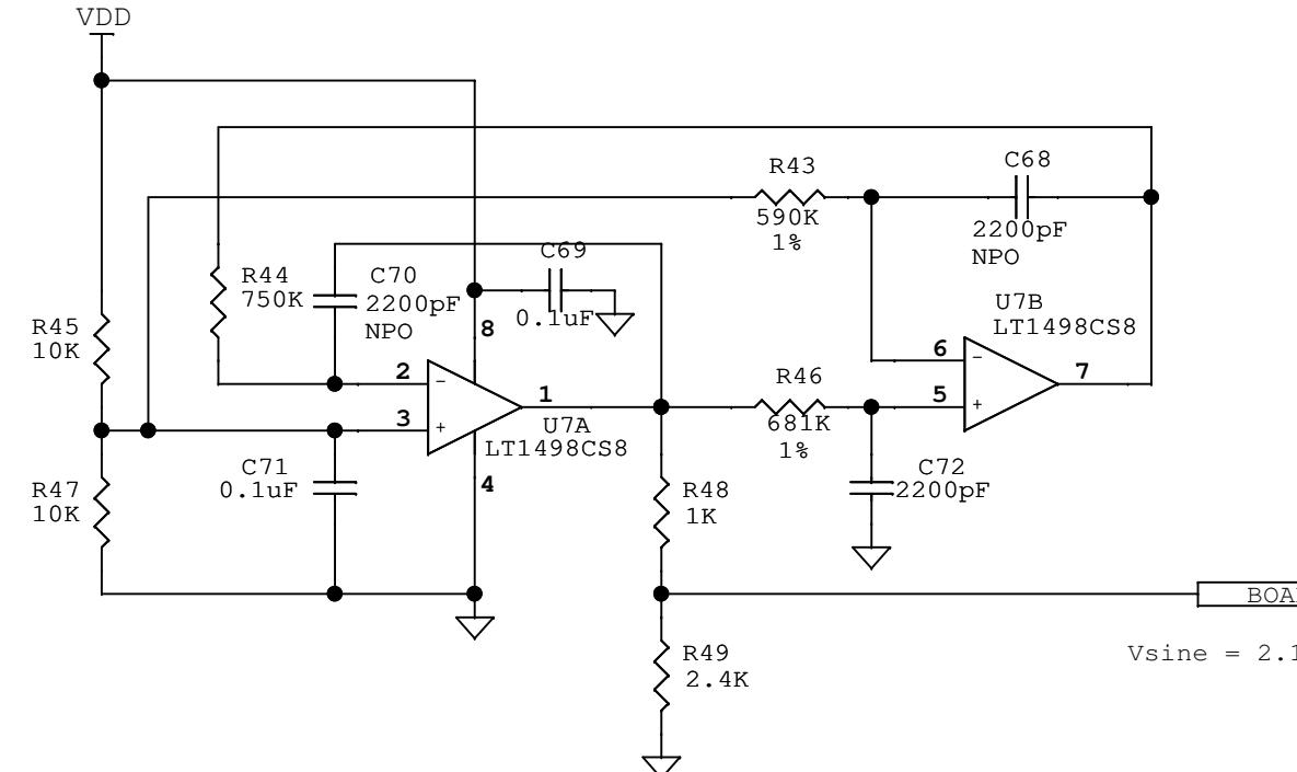
$V_{\text{sin}} = 2.1\text{Vpp}, 1.2\text{Vos}, 105\text{Hz}$
