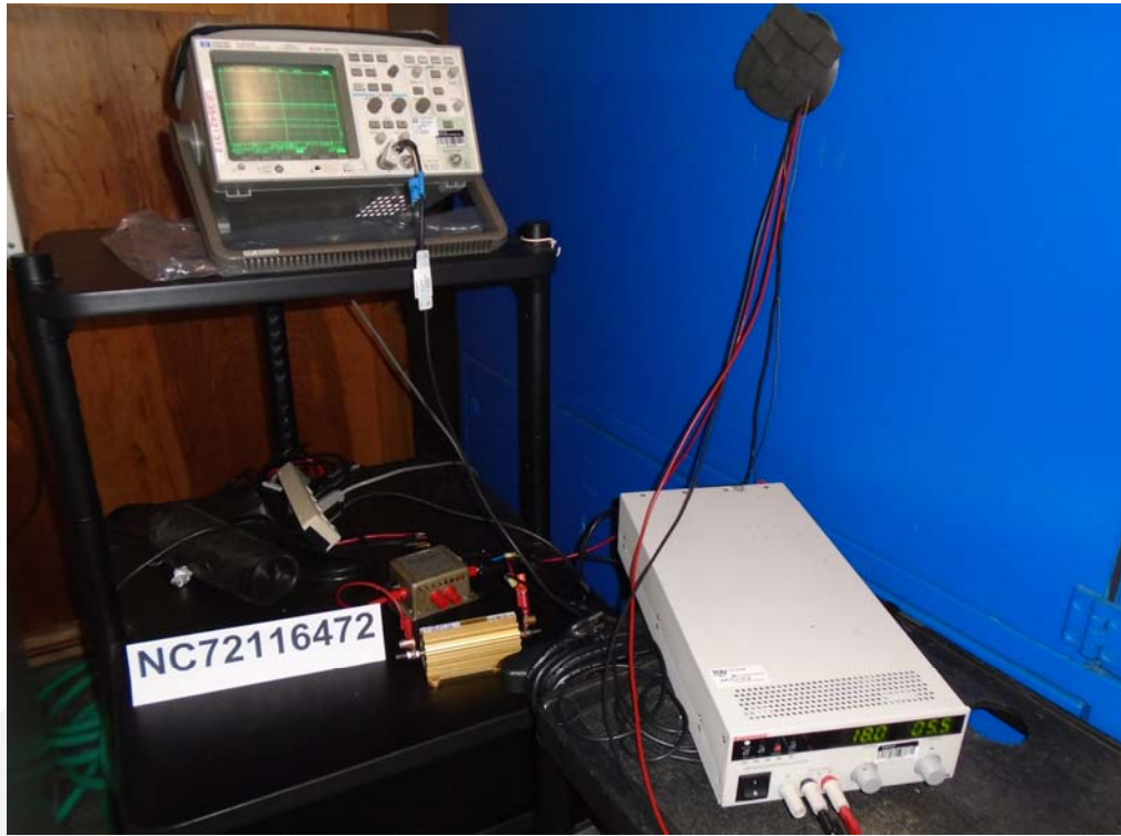
Test-setup photo(s): ISO 16750-2: 2012 - Clause 4.3 - Overvoltage
