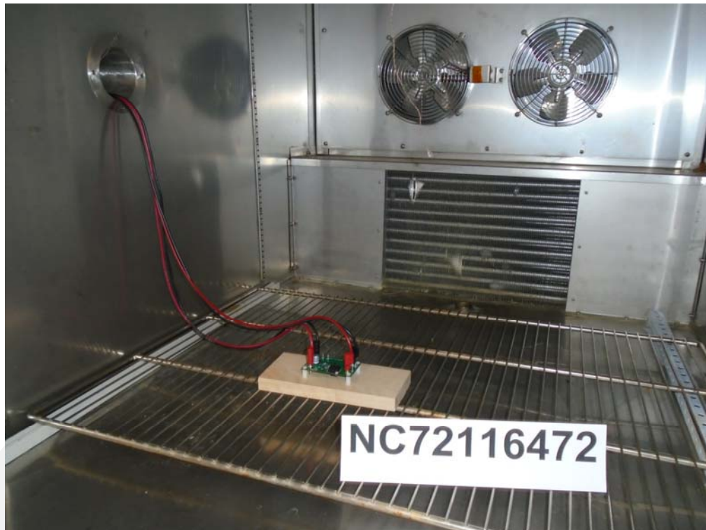
Test-setup photo(s): ISO 16750-2: 2012 - Clause 4.3 - Overvoltage
