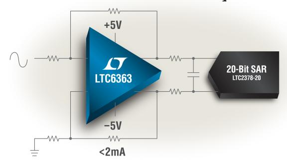
Drive your precision ADC with the power efficient LTC $^{\circ}$ 6363. Drawing just 1.9mA, this fully differential amplifier achieves 100µV max input offset voltage and 2.9nV/ $\sqrt{\text{Hz}}$  broadband noise. With a 2.8V to 11V supply range and rail-to-rail outputs, the LTC6363 is well matched to the ADC's full range, to achieve maximum signal path performance.
