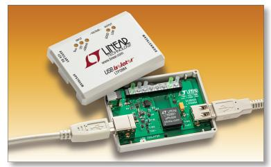
The LTPTM2884 is a complete  $2500V_{RMS}$  inline USB isolator based on the LTM2884 and features a rugged enclosure with high retention USB connectors, hot plug protection, surge/ESD protection and LED status indicators. No drivers or software are required, just plug and play.
