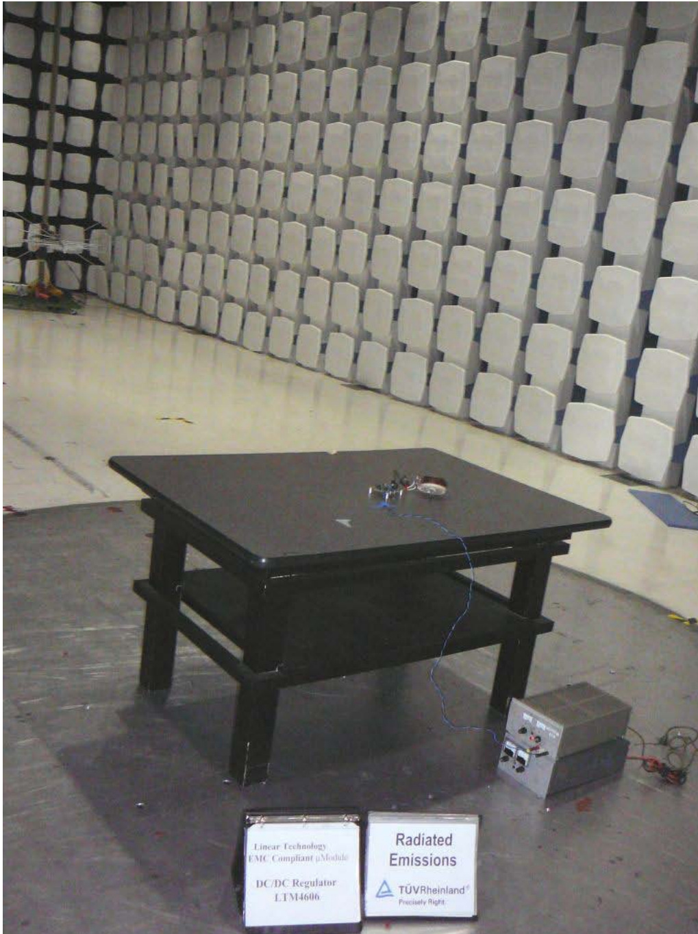
Figure 4 – Radiated Emissions 30 - 1000 MHz Test Setup – Back
