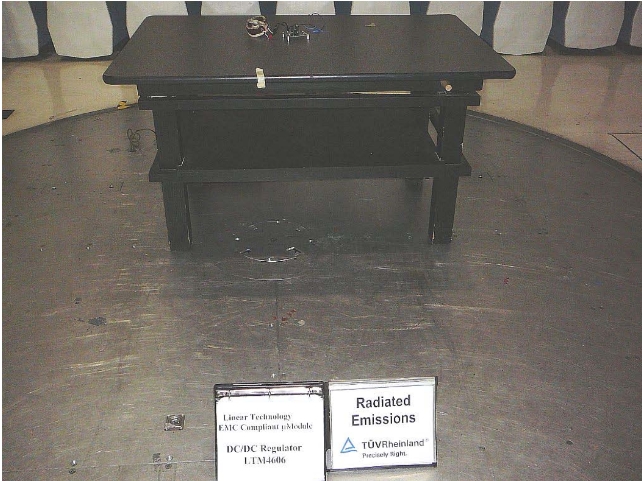
Figure 3 – Radiated Emissions Test Setup – Front
