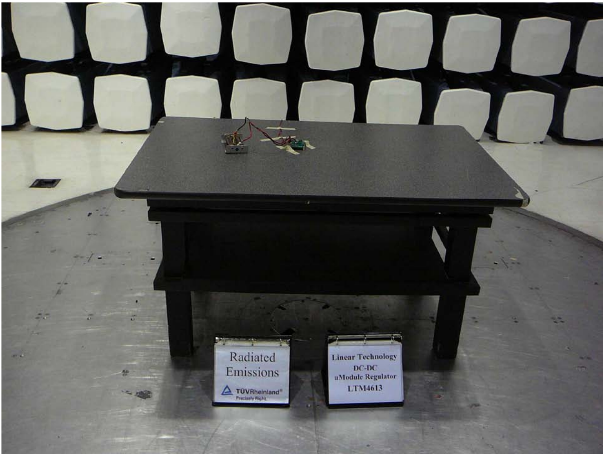
Figure 3 – Radiated Emissions Test Setup – Front
