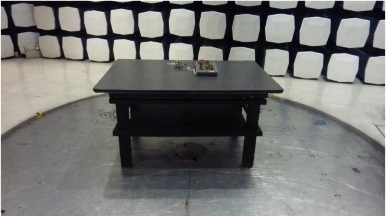
Figure 4 - Radiated Emissions Test Setup 30 - 1000 MHz - Front
