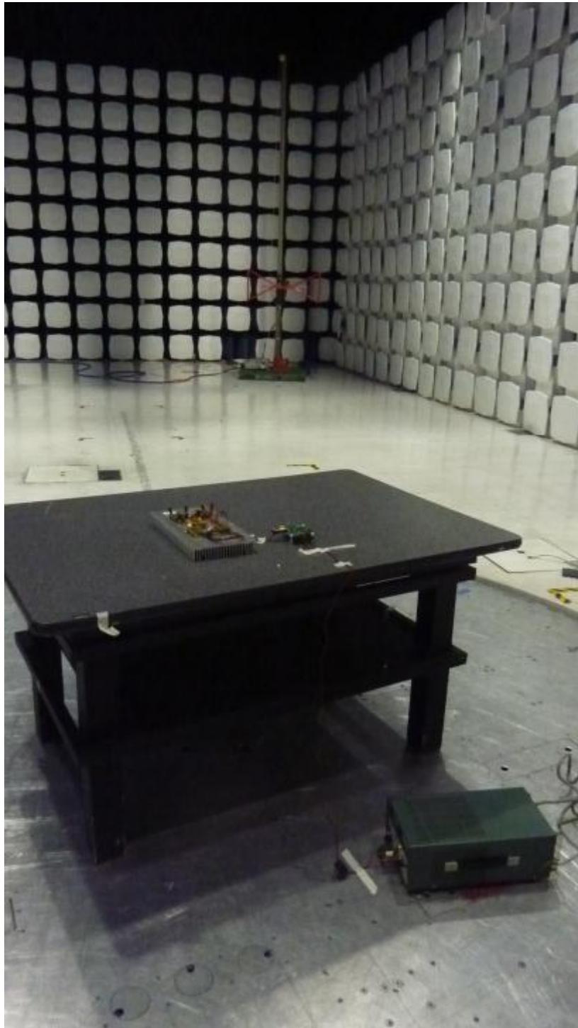
Figure 5 - Radiated Emissions Test Setup 30 - 1000 MHz - Back
