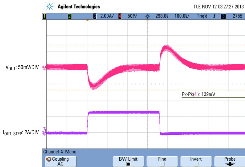
Figure 6. Measured Channel 2 Load Transient V_{IN} = 12V , V_{OUT1} = 3.3V , I_{STEP} = 0A to 2.5A I_{STEP} Slew Rate = 1A/\mu s
