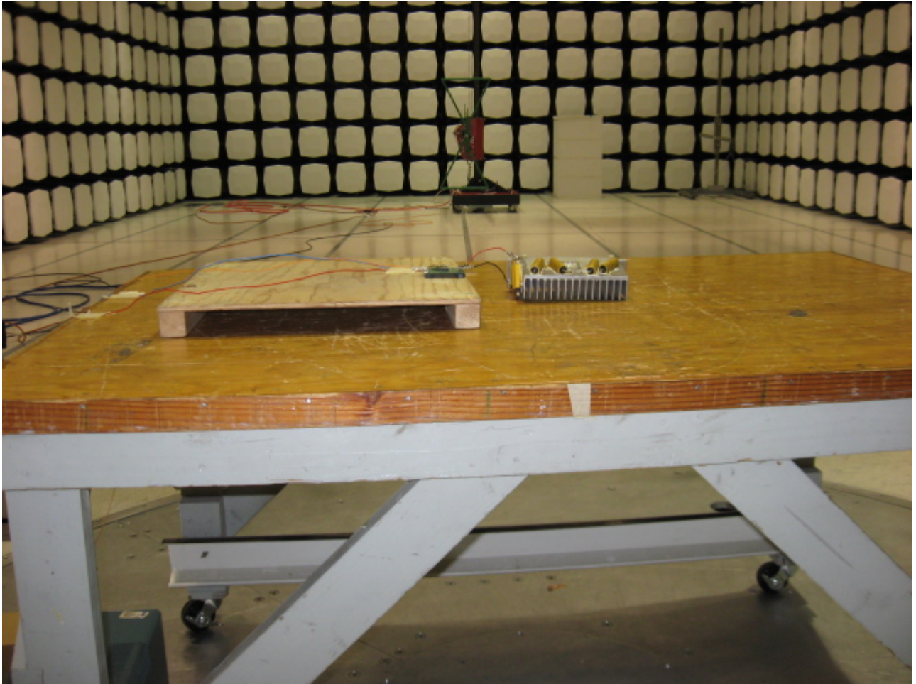
Photograph 1. Radiated Emission: Limits of Electromagnetic Radiation Disturbance, Test Setup
