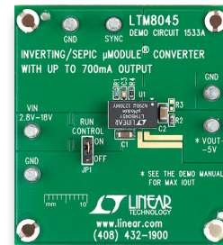
DC1533A: LTM8045 Demo Board 2.8V to 18V IN , 5V or -5V OUT
