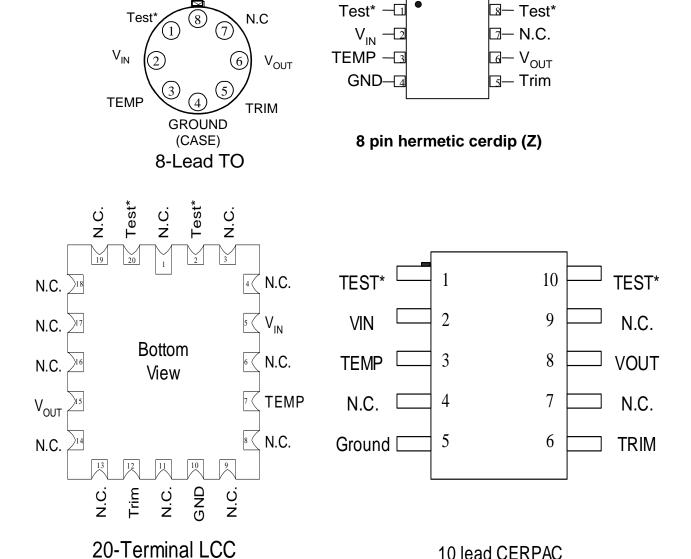
Figure 1 - Terminal connections. \* Reserved for factory testing. Make no electrical connection to these pins.
