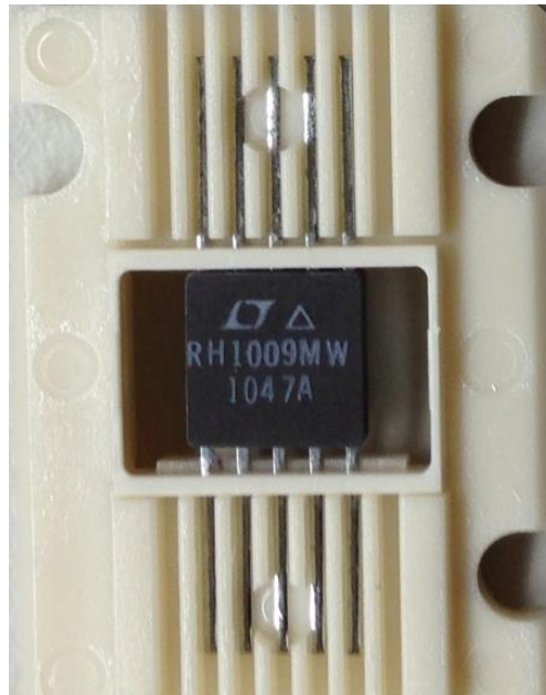
Figure A1: Top View showing part number and date code
