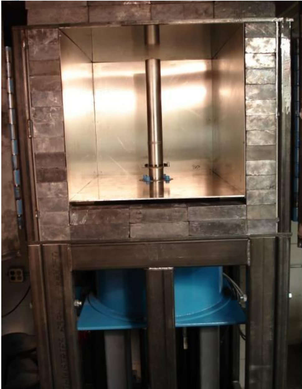
Figure 2.1. Aeroflex RAD's high dose rate Co-60 irradiator. The dose rate is obtained by positioning the device-under-test at a fixed distance from the gamma cell. The dose rate for this irradiator varies from approximately 300rad(Si)/s close to the rods down to 1rad(Si)/s at a distance of approximately 2-feet.
