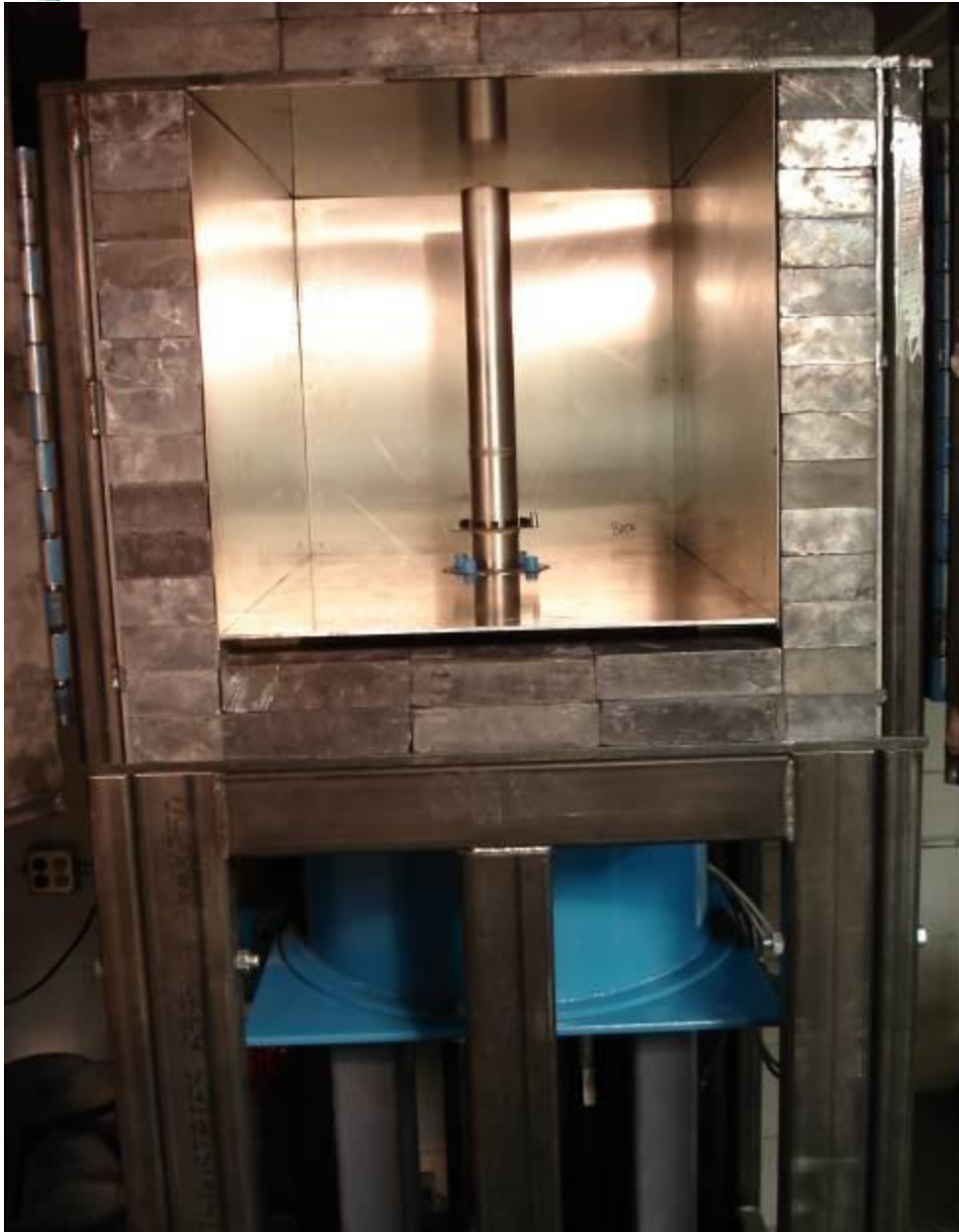
Figure 2.1. Aeroflex RAD's high dose rate Co-60 irradiator. The dose rate is obtained by positioning the device-under-test at a fixed distance from the gamma cell. The dose rate for this irradiator varies from approximately 120rad(Si)/s close to the rods down to 1rad(Si)/s at a distance of approximately 2-feet.
