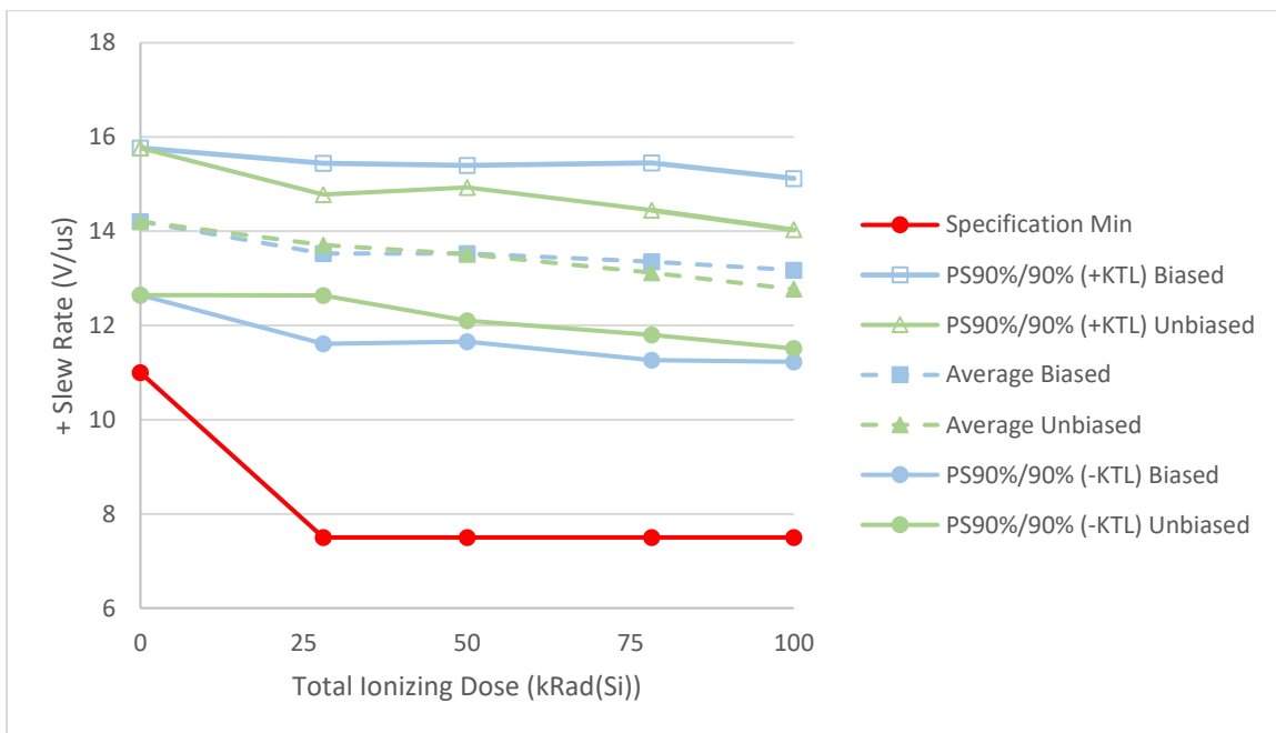
Figure A-6. + Slew Rate vs. TID for the RH1028M irradiated at low dose rate.
