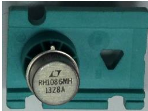
Figure A1: Top View showing ID and Date Code
