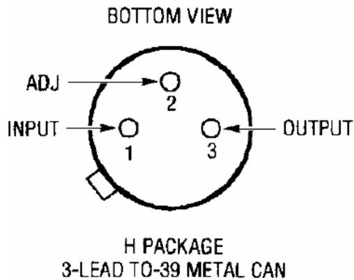
Figure B.2. H package drawing (for reference only). This figure was extracted from the LINEAR TECHNOLOGY RH117 Datasheet.
