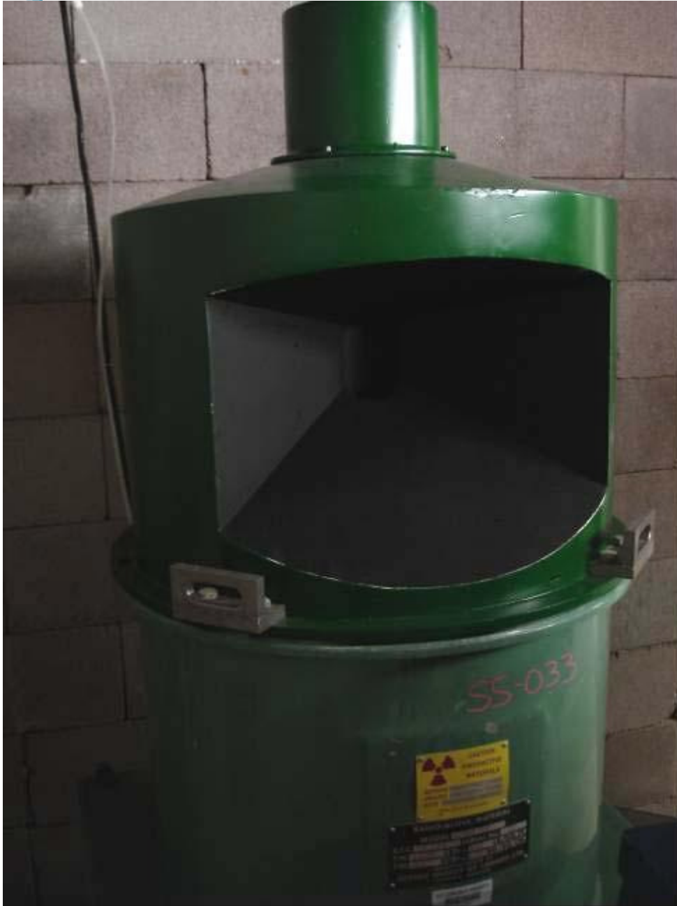
Figure 2.1. Aeroflex RAD's Co-60 irradiator. The dose rate is obtained by positioning the device-under-test at a fixed distance from the gamma cell. The dose rate for this irradiator varies from approximately 50rad(Si)/s close to the rods down to <1mrad(Si)/s at a distance of approximately 4-meters.
