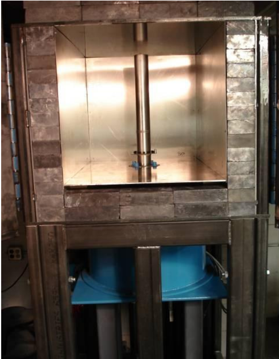
Figure 2.1. Radiation Assured Devices' high dose rate Co-60 irradiator. The dose rate is obtained by positioning the device-under-test at a fixed distance from the gamma cell. The dose rate for this irradiator varies from approximately 120rad(Si)/s close to the rods down to 1rad(Si)/s at a distance of approximately 2-feet.
