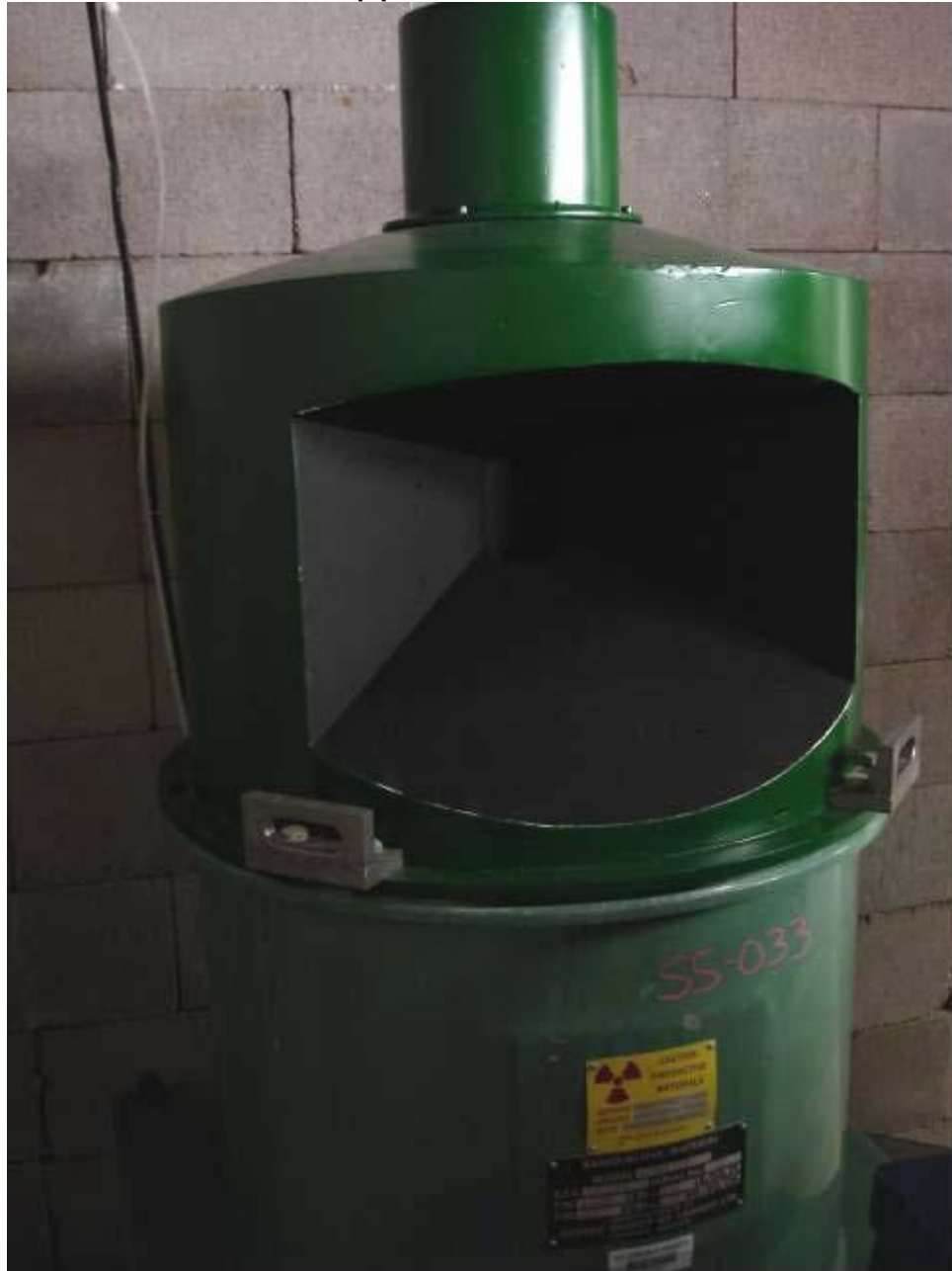
Figure C1: Cobham RAD's ^{60}\text{Co} irradiator. The desired dose rate is obtained by positioning the device-under-test at a fixed distance from the gamma cell. The dose rate for this irradiator can vary from approximately 50rad(Si)/s, at a position close to the rods, down to <math><1\text{mrad(Si)/s}</math>, at a distance of approximately 4-meters from the rods.
