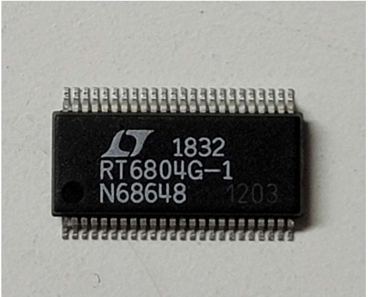
Figure 2. Photograph of a RT6804HG-1 G Package 48 Lead SSOP.
