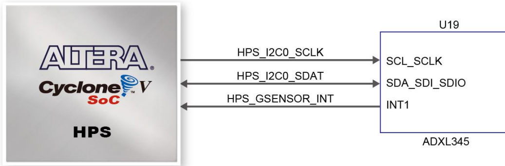
Figure 3-28 Connections between HPS and G-Sensor device.
