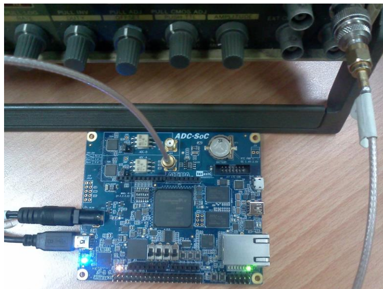
Figure 4-6 Hardware setup for the HIGH-SPEED-ADC
