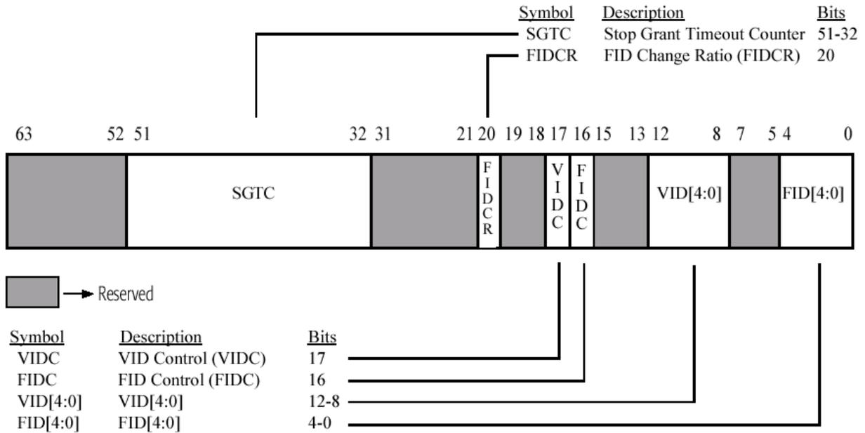
Figure 1. FidVidCtl Register - MSR C001\_0041h
