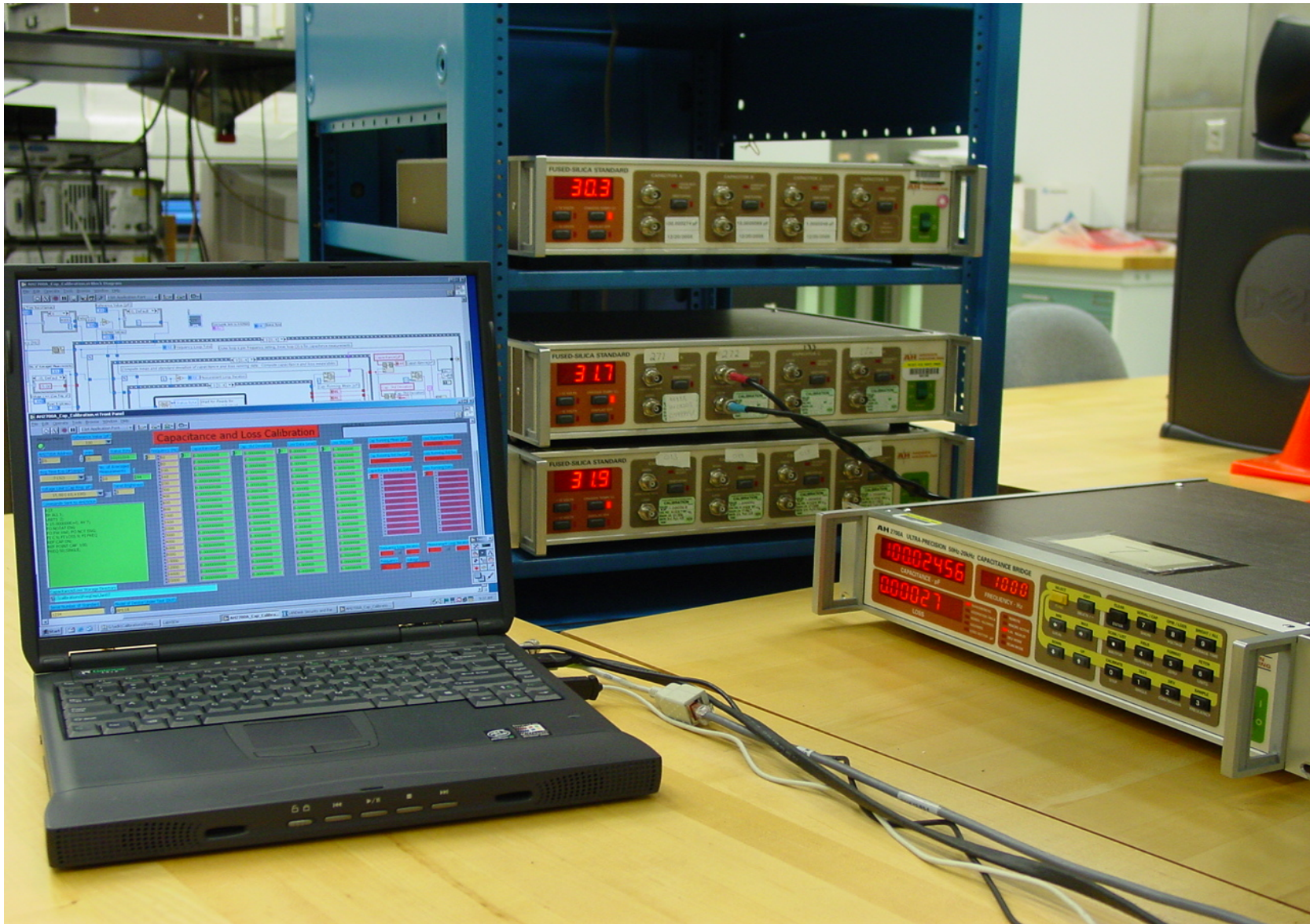
Fig. 9. Photograph of the capacitance bridge, controlling laptop, and reference and customer fused-silica standard capacitors.
