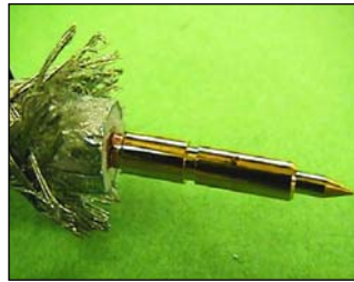
Figure 6 · Properly soldered cable end.
