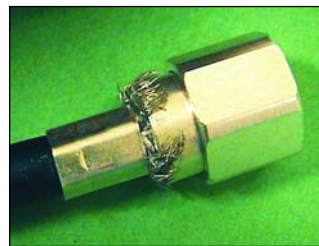
Figure 8 · Improperly attached connector.
