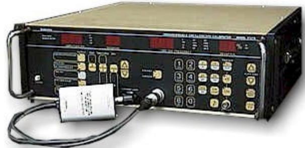
**Volts/Division Mode** (Used for calibration of vertical display accuracy and attenuator compensation)
