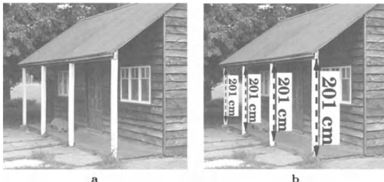
Fig. 5.1. Measuring distances of points from a reference plane (the ground) in a single image: a the four pillars have the same height in the world, although their images clearly are not of the same length because of perspective effects; b as shown, however, all pillars are correctly measured to have the same height.
