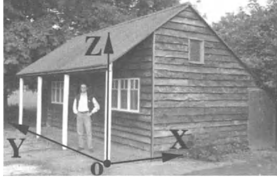
Fig. 5.13. Computing the location of the camera: equations (5.18) are used to obtain: X_c = -381.0 cm, Y_c = -653.7 cm, Z_c = 162.8 cm.
