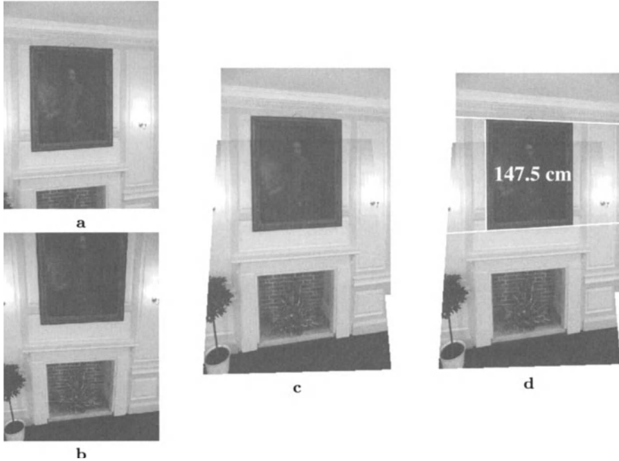
Fig. 4.16. Mosaicing two images: a and b original images of The Queen’s College Middle Common Room (MCR), Oxford; the two images are taken from the same viewpoint, just rotating the camera (no parallax effect); c mosaic image; d mosaic with measurements superimposed.
