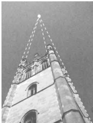
Fig. 3.11. Computing the vanishing point of the vertical direction: images of parallel edges of the tower (Magdalen College, Oxford) intersect in the vanishing point (white circle); only two such lines are sufficient.
