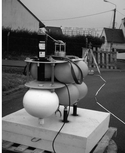
Figure 3.9. Example of a cage used for moorings placed on the sea bed. In the foreground, we can see a Nortek AquaPro Doppler current meter; in the middle, an acoustic release; and at the bottom buoys to allow the cage to rise when the release system is activated and a concrete weight held by the release system (Courtesy of © SHOM)
