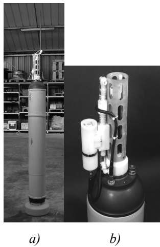
Figure 3.19. a) An APEX float with a conductivity sensor on its upper side. At the base, we can see the mechanical system used to adjust its buoyancy (courtesy of © SHOM). b) Head of an APEX buoy equipped with Sea Bird temperature–conductivity sensors and a Clark polarimetric dissolved oxygen sensor (Courtesy of S.C. Riser, Univ. of Washington)
