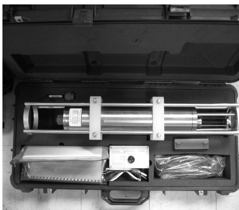
Figure 2.34. The Valeport MIDAS SVP model sound velocity profiler in its transport case, with interface box used to recharge its batteries and extract memorized data (Courtesy of © SHOM)
