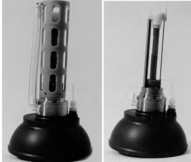
Figure 2.28. Fixture made by Sea Bird Engineering, Inc. in order to adapt a conductivity cell and a temperature probe to drifting floats. The outfit is called SBE 41. In the photo on the left, the cell is protected by a guard. The exterior TC-duct enables water to circulate through pumping in order to align the response time of the temperature sensor and that of the conductivity cell. The “U” fixture enables conservation of water in the cell while the buoy returns to the surface. This avoids salt and different pollutants from being deposited. The cell drift is therefore better managed (Courtesy of Sea Bird Electronics, Inc.)
