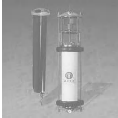
Figure 2.35. A Nortek Aquadopp acoustic current meter and a MORS MC 3X0 rotor (Courtesy of Oceano Technologies)
