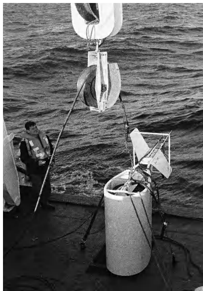
Figure 4.8. Launch of a low-frequency transducer used for tomographic experiments where the acoustic source is towed (Courtesy of © SHOM).
