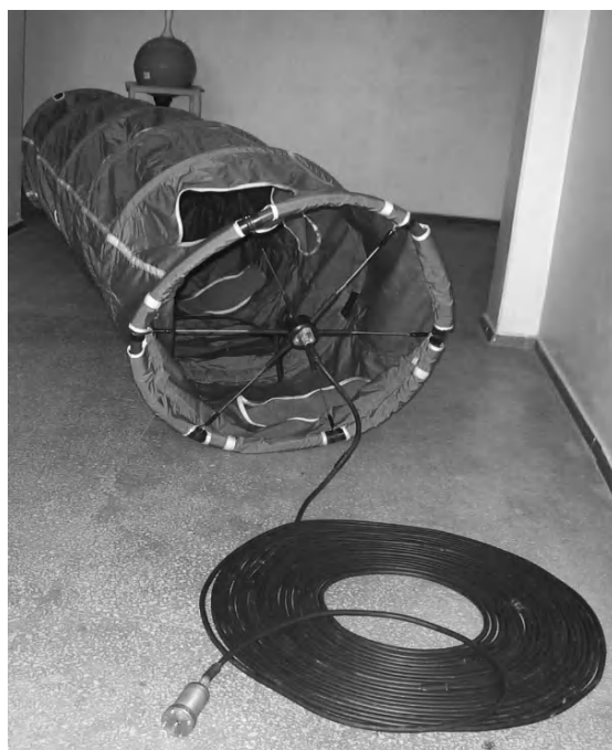
Figure 3.14. A holey socks floating anchor connected to a thermistor chain. In the background, we can see an surface velocity profiler-type surface buoy (Courtesy of Marlin-Yug, Sebastopol, Ukraine)
