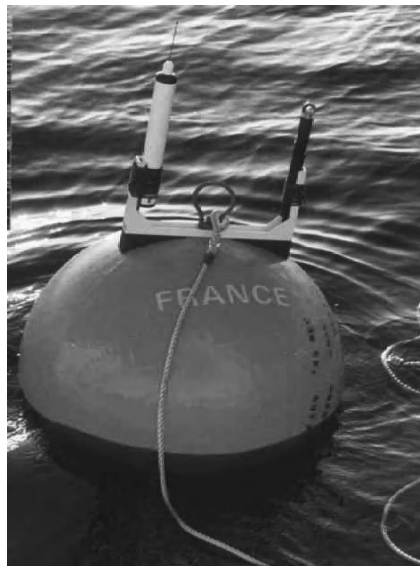
Figure 3.12. Surface buoy equipped with a flash lamp (Courtesy of © SHOM)
