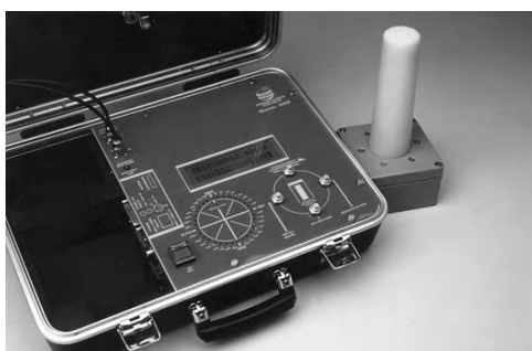
Figure 2.52. Gonio SERPE-IESM 400P receiver with antenna, enabling localization of drifting buoys (Courtesy of SERPE – IESM). Newer, equivalent systems have been commercialized by Doppler Systems LLC
