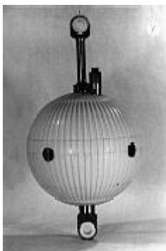
Figure 2.39. Example of the S4 electromagnetic current meter produced by InterOcean Systems, inc. It is a sphere that contains four electrodes (black dots) and a frame that enables its suspension from a mooring line (Courtesy of InterOcean Systems, Inc)
