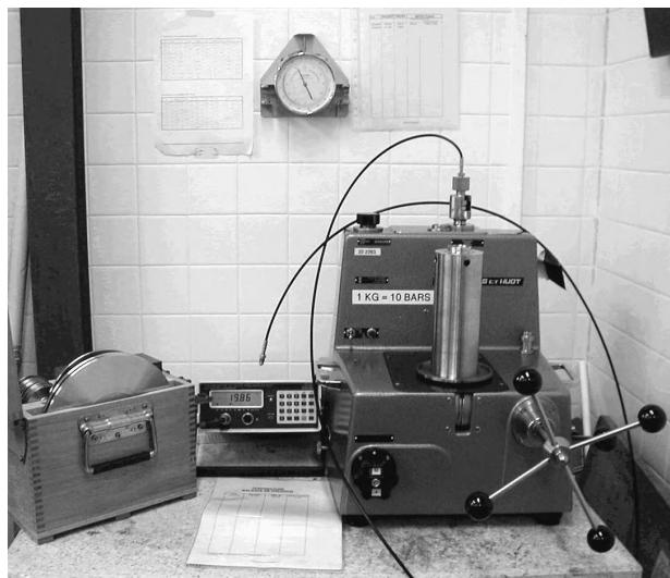
Figure 1.7. A dead weight tester with its flexible pipe allowing linkage to the sensor to be calibrated, its temperature gauge to correct for piston-cylinder expansion, and its calibrated mass box (© SHOM)
