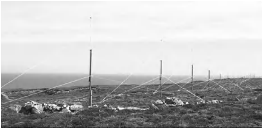
Figure 2.66. Example of an installation of receiver antennas of a WERA-type system (Courtesy of © SHOM)
