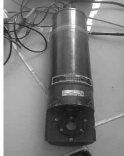
Figure 2.73. The Aquatracka fluorimeter III produced by Chelsea Instruments (© SHOM)
