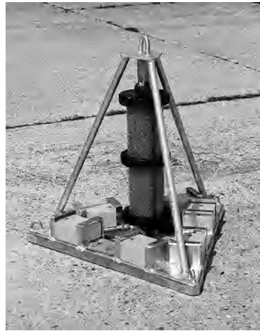
Figure 2.62. Example of submerged pressure sensor tide gauge (SLS 23 by Mors) installed in a ballasted cage (Courtesy of © SHOM)
