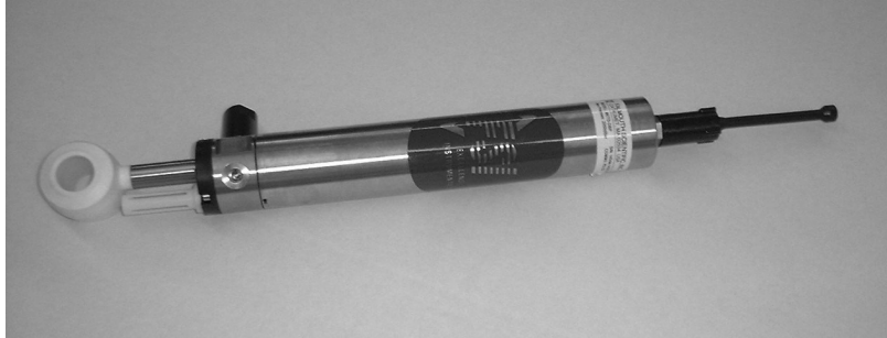
Figure 2.26. Example of an inductive sensor attached to a CTD probe (Courtesy of FSI, Inc.)
