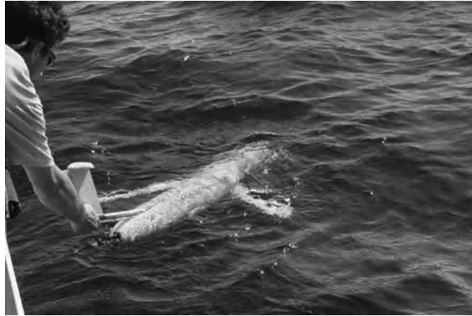
Figure 4.10. Launching of a prototype glider (Courtesy of © SHOM – ENSIETA)
