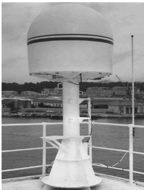
Figure 3.6. INMARSAT radome antenna (Courtesy of © SHOM)
