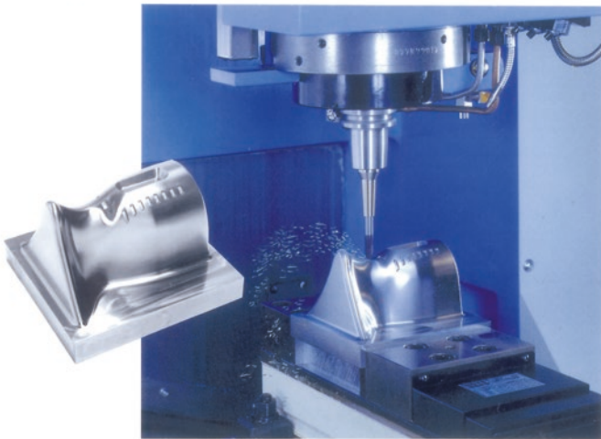
Specification: X-axis travel: 4200 mm; Y-axis travel 1400 mm; Z-axis travel 585 mm; Rapid traverse 120 m min -1 ; Feedrate 40 m min -1 ; Spindle speed 18,000 rev min -1 ; Spindle power 37 kW; Tool spindle type CAT#50; Tool storage capacity 60 tools.
