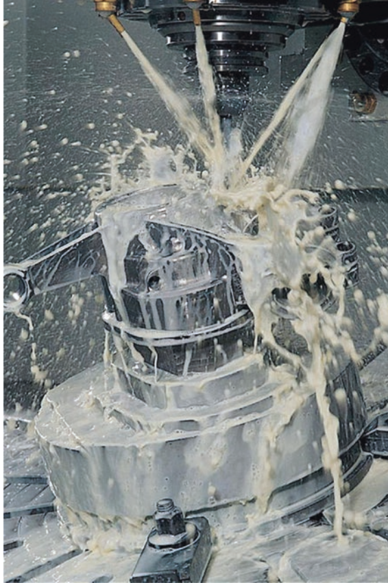
Flood-coolant utilised to flush away any chips [courtesy of Fuchs Lubricants (UK) Plc]
