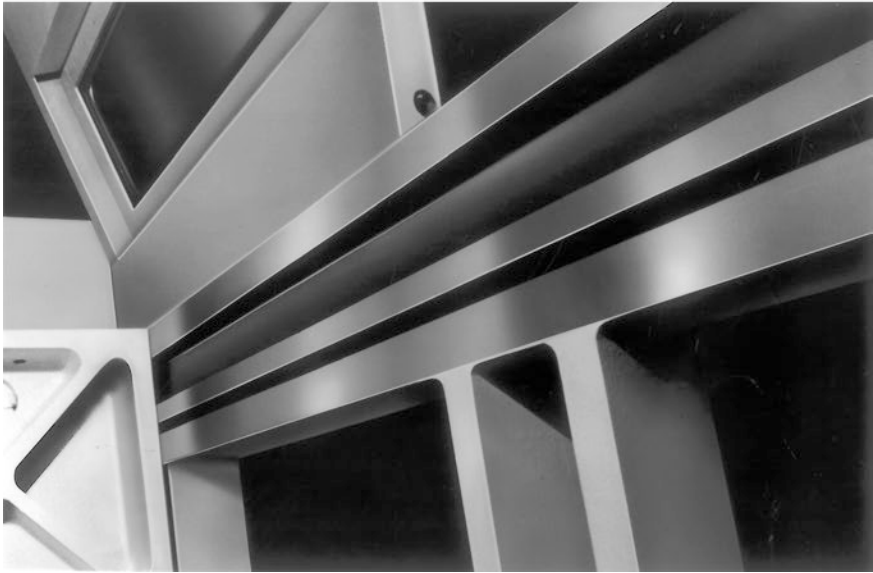
Fig. 1.36 The partial assembly of a slant-bed turning centre, having a box-like ribbed cast iron structure, with hardened ways (courtesy of Cincinnati Machine UK Ltd.)
