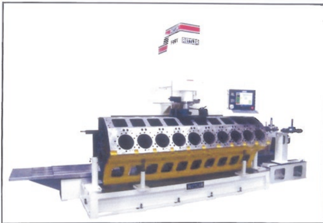
A Travelling Column CNC (Vertical) Boring Machine, machining a V20 engine block.
