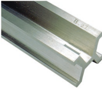
The basic mechanical design and the geometric construction shape of the International Prototype Metre—circa 1889
