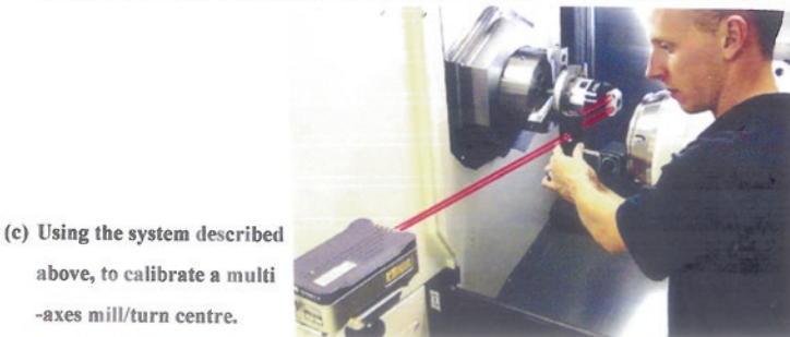
Fig. 2.14 Typical images of multi-axes laser calibration of machine tools (courtesy of Reinshaw plc)
