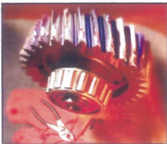
Fig. 6.13 Bearing and gear corrosion in machine tools [source Kuhnell, B.T. (Monash University, Australia) 2004]
