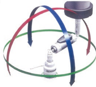
Both partial arcs & circular motions can be achieved in a number of differing three-dimensional planes, typically: X-Y, X-Z, & Y-Z
