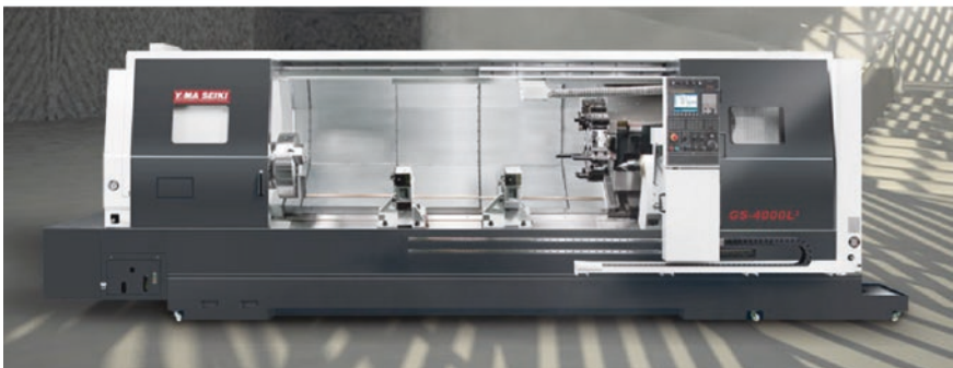
Heavy-duty Turning Centre, 30 degrees slant bed with wide box ways, with 2-speed head stock driven by a 37 kW, powerful Z-axis spindle motor, the axes rapids are 24 m/min. on X and Z axes, with FANUC motors and control.
