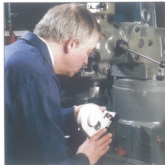
Fig. 3.16 Typical clinometer designs—utilised for either angular positional axis setting or work-piece checking (courtesy of Spectrum Metrology)
