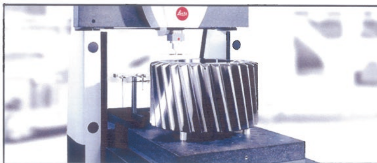
(b) Fixed bridge/moving table-type CMM : Leitz PMM-C – is versatile, but ultra-high precision CMM and gear metrology-checker.
