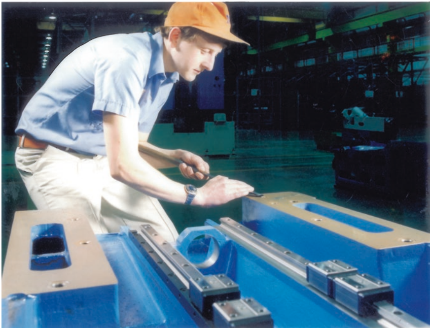
Fig. 1.37 The 'traditional' scraping technique for production of flat surfaces—which then reduces potential 'high-spots' on the casting's surface, while imparting a good lubrication surface condition on a machine tool's 'meehanite cast iron' base element, minimising 'stick-slip' for its moving members [courtesy of Yamazaki Mazak Corporation (Worcester, England)]
