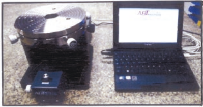
An ultra-precision air-bearing rotary table, with sub-arc rotational position capabilities.
