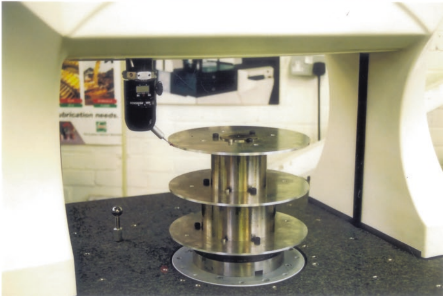
Fig. 5.20 An CMM inspection procedure of the machinable disks in situ on the stereometric artefact [after: Smith et al. (2001)]
