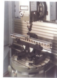
(c) Step Gauge shown lying horizontally aligned along the X-axis of the CNC machine's rotary table, equipped with Touch-trigger Probing:
