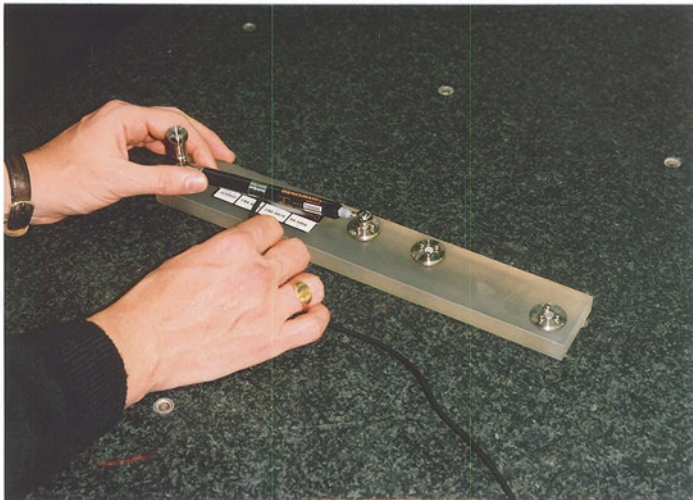
Fig. A.25 The Ballbar portable case and Zerodur™ calibrated artefact—for variable length calibration (courtesy of Renishaw plc)
