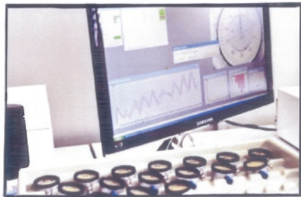
Dial gauge calibration – calibration with a 'deviation diagram and 'error' for ingoing-and-outgoing plunger motion, repeatability and hysteresis, according to DIN 878. [Courtesy of Käfer Messuhrenfabrik GmbH & Co. KG]
