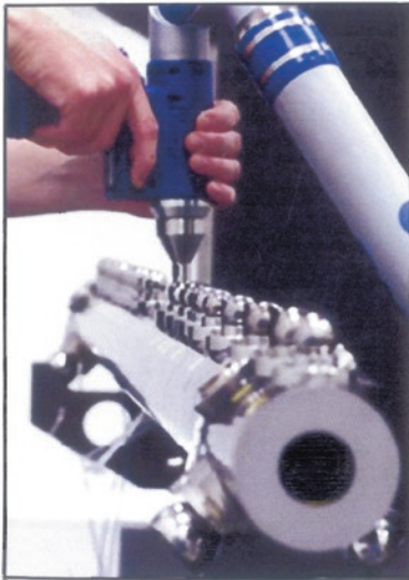
Calibrating an 'Articulated arm', by utilising a previously referenced and calibrated artefact.
