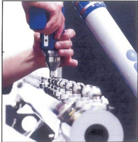
Fig. 5.28 An 'articulated arm CMM' prior to use, requires verification against a calibrated artefact [courtesy of the National Physical Laboratory (UK)]
