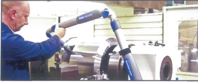
Inspecting critical dimensional features of an accurate & precise turned component employing an 'articulated arm'. [Courtesy of FARO Technologies Inc]
