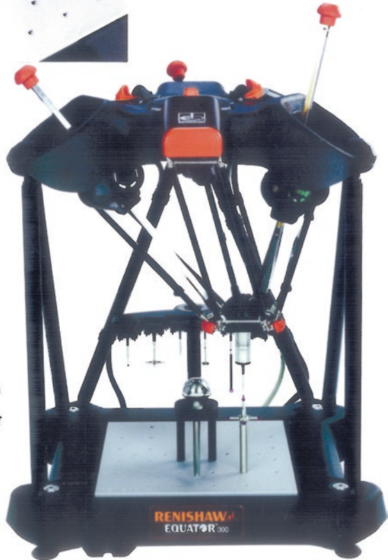
Fig. 5.26 The parallel kinematic mechanism-based machine: equator™, that can complete in terms of both: speed of operation and versatility, with 'hard-gauging' techniques (courtesy of Renishaw plc)
