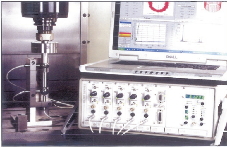
A 5-sensor Spindle Error Analyser being utilised on a vertical Machining Centre, with the instrument's measurements conforming to ISO 230-3/7 Standards.
