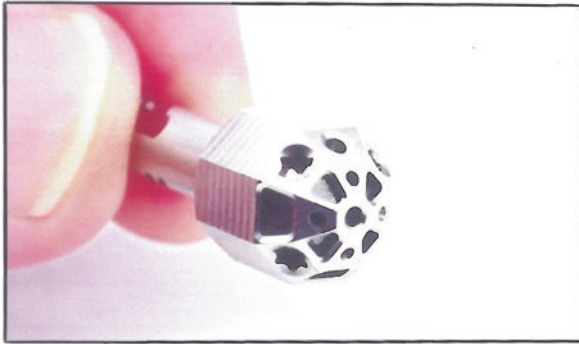
A micro-machined prismatic part, after machining on a 5-axis Micro Milling Platform. [Courtesy of Microlution, Inc. (Chicago, USA)]
