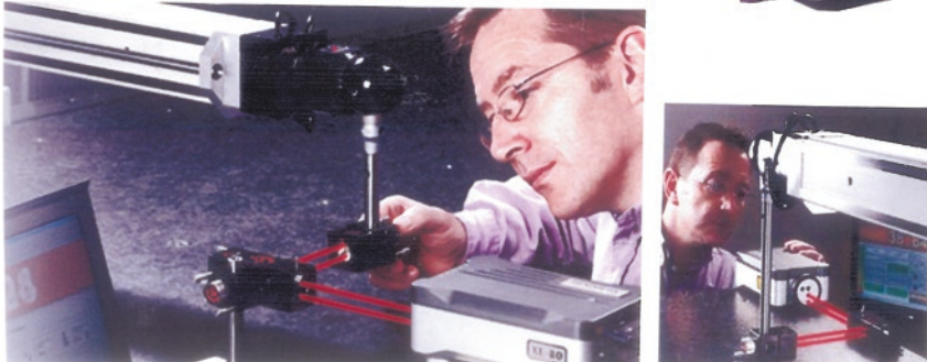
(c) Laser mounted directly onto the cantilevered CMM's table, adjusting the optics, prior to calibration.
