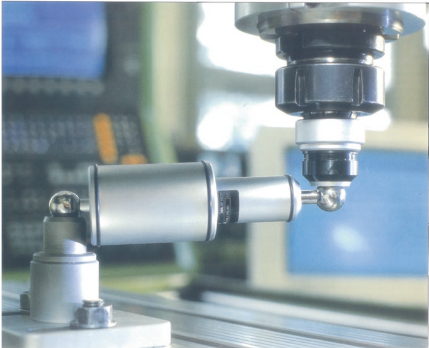
Fig. 4.7 The double acting ballbar on the table of a CNC machine tool (courtesy of Heidenhain (G.B.) Ltd.)
