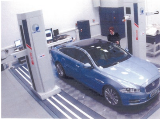
A large-scale Twin Column (LK) CMM – with Horizontal Scanning Arms, equipped with Digital Cross-scanner/laser for Reverse Engineering comparison/validation.
