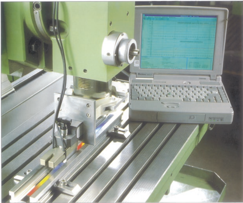
A typical setup for calibrating alignments on CNC machine tools up to 1000 mm, with a Linear Comparator System.
