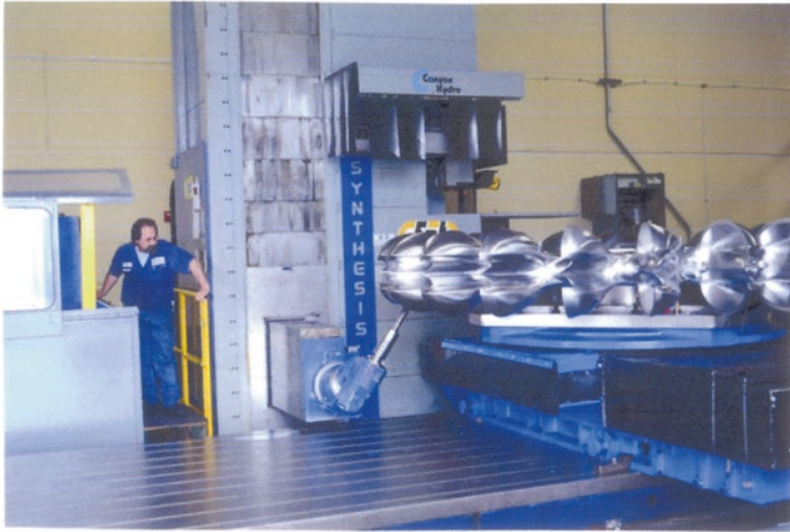
(a) The machining of a large Hydro-impeller situated on an integral rotary table on the Travelling Column CNC Milling Machine. [Courtesy of Canyon Hydro (Deming, WA, USA)]
