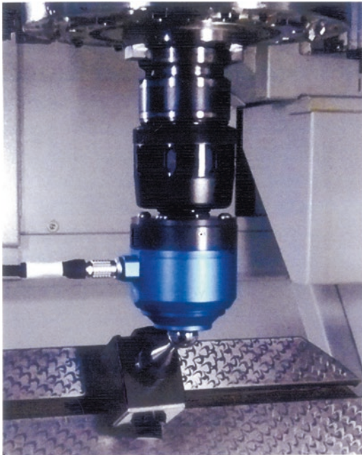
5-axis Rotary Analyzer System (i.e. 'R-test') on a Machining Centre. [Courtesy of IQL, East Hartford, CT (USA)]
