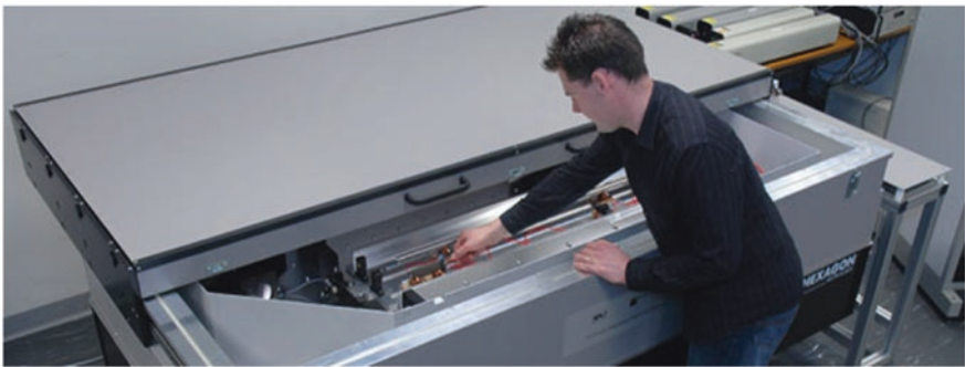
The NPL-designed/hexagon metrology manufactured (LBI1.5)—length bar interferometer (courtesy of The NPL/Hexagon Metrology)
