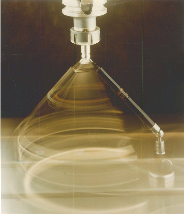
Fig. A.27 The ‘dynamic’ Ballbar assessment of a vertical machining centre at an inclined plane (courtesy of Renishaw plc)
