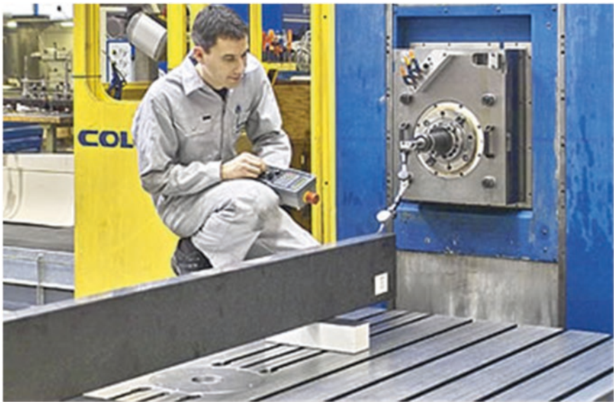
Utilising a calibrated granite Straightedge for inspection of a Horizontal Machining Centre's linear axis (courtesy of Kunz Precision AG, Zofingen, Switzerland)
