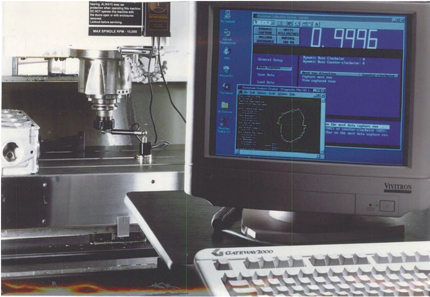
Fig. A.28 Quick Ballbar calibration/diagnostic assessment of a vertical machining centre—with workpiece in-situ, prior to subsequent machining (courtesy of Renishaw plc)
