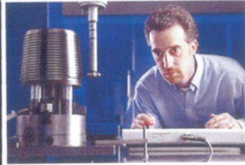
The Dimensional Measurement Services project provides industry high accuracy dimensional measurements within an internationally accepted quality system. Here, measurement of API Rotary Master Gauge on CMM. [Courtesy of The National Institute of Standards and Technology (NIST)]
