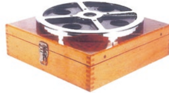
Coventry Gauge & Tool Matrix's 72-sided Mirror polygon , having a cumulative angular spread: +16,3/-5,9 arc seconds (Ø300 mm). [Courtesy of Hofstra Group, Ltd. Co. (NM, USA)]
