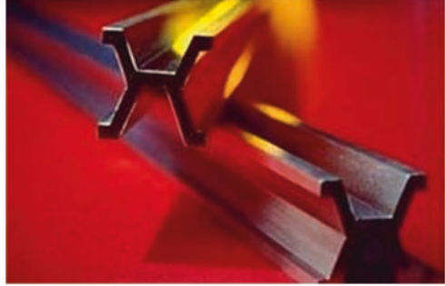
The basic mechanical design and the geometric construction shape of the International Prototype Metre—circa 1889
