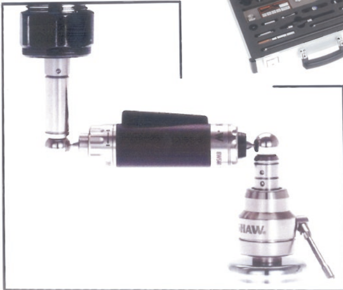
Fig. 4.3 A ‘wireless ballbar’ for the quick and efficient ‘health checking’ of a CNC machine tool (courtesy of Renishaw plc)
