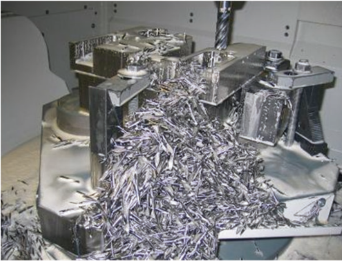
High volume of swarf generated by the CNC machine [courtesy of SolidCam Inc. (Newtown, PA, USA)]
