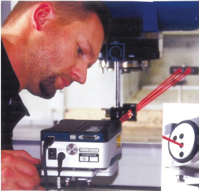
a) Setting up the calibration of a vertical Machining Centre – Laser tripod mounted.
