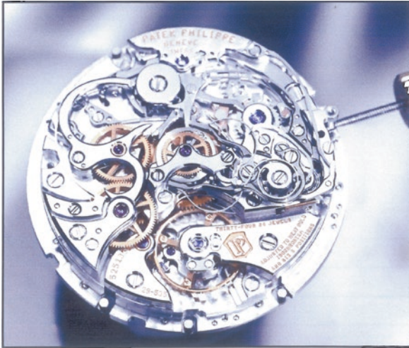
Micromachining to a positional accuracy of \leq \pm 1 \mu\text{m} . [Courtesy of Cadence Inc. (USA)]
