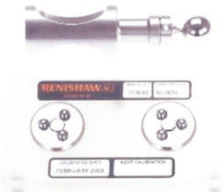
Part of the Small Circle Accessory Kit (i.e. 50 mm): the calibration fixture being made from Zerodur™ , for the task of calibrating the Small Circle Adaptor prior to use.
