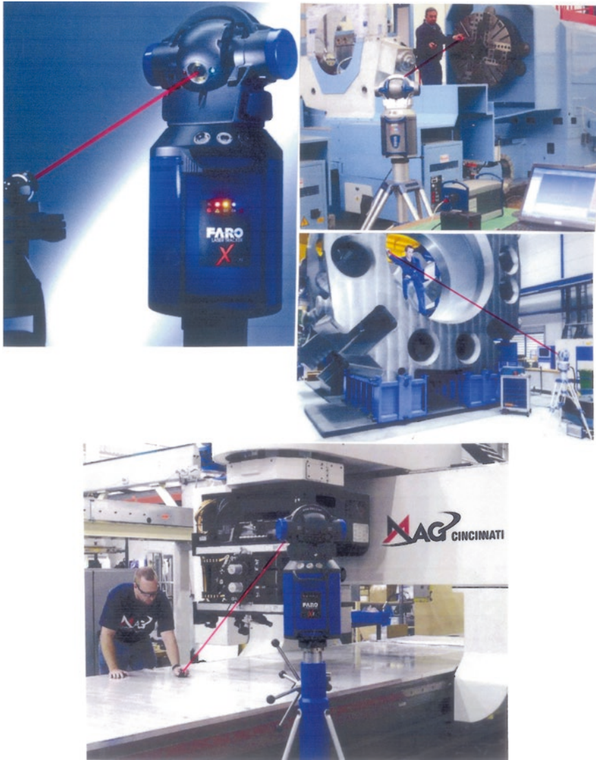
Fig. 2.18 Laser tracker applications can be wide-ranging in their inspection/calibration applications (courtesy of FARO Technologies Inc)
