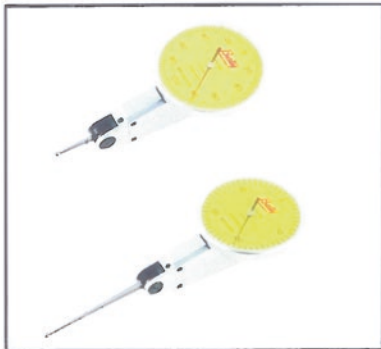
(b) A mechanical Dial Test Indicator (DTI) – used to verify / calibrate machine tools.
