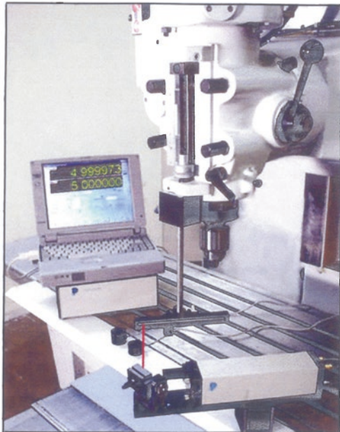
(b) A 'Laser/Ball-bar' circular test being conducted on a CNC Turret mill.
