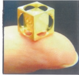
Micromachining to a positional accuracy of \leq \pm 1 \mu\text{m} . [Courtesy of Cadence Inc. (USA)]
