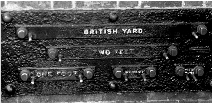
Figure 1.1 Early dimensional standard at the Royal Observatory, Greenwich, England. (Photo by Graeme C. Payne.)
