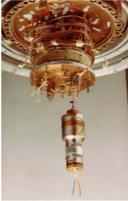
Fig. 7. – NPL stainless-steel triple-point cell suspended in the cryostat.
