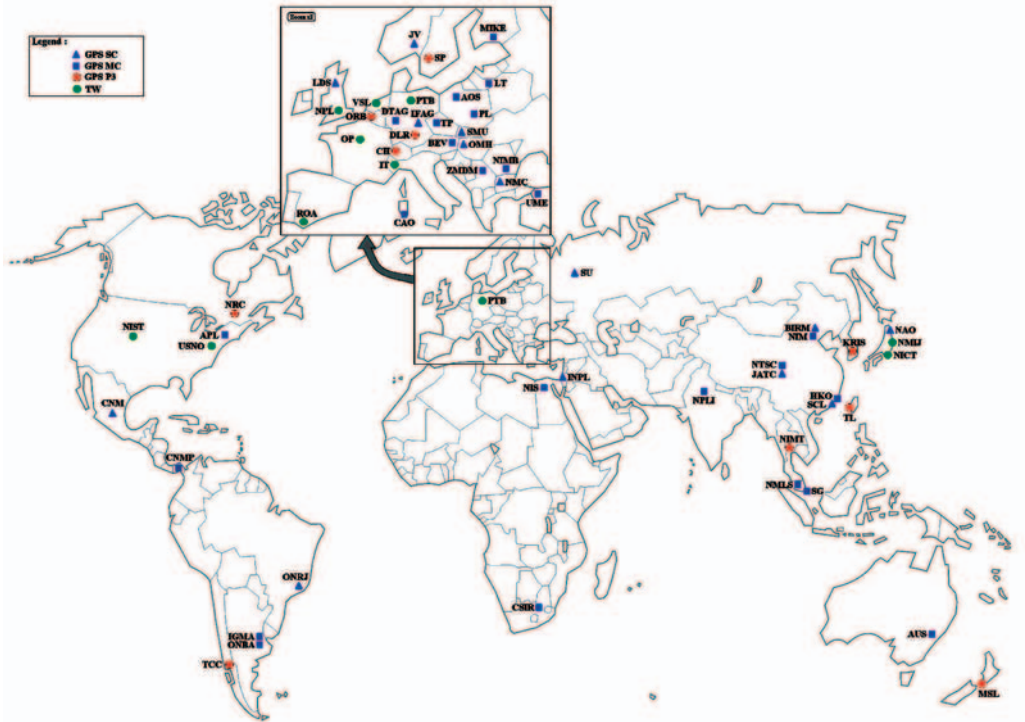
Fig. 3. – Laboratories participating to the calculation of timescales at the BIPM as in October 2006. Laboratories operating GPS equipment are compared to the PTB; laboratories equipped with TWSTFT stations in Europe and North America are compared to the PTB; those in the Asia-Pacific region are compared to NICT.
