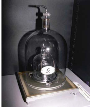
Fig. 1. – The international prototype of the kilogram.
