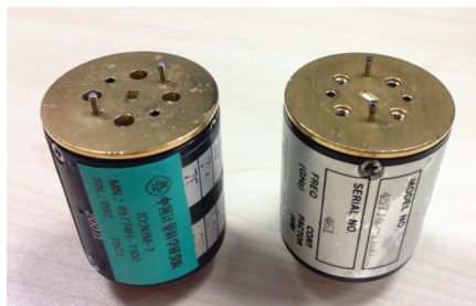
Figure 3. One popular type of waveguide thermistor mount.
