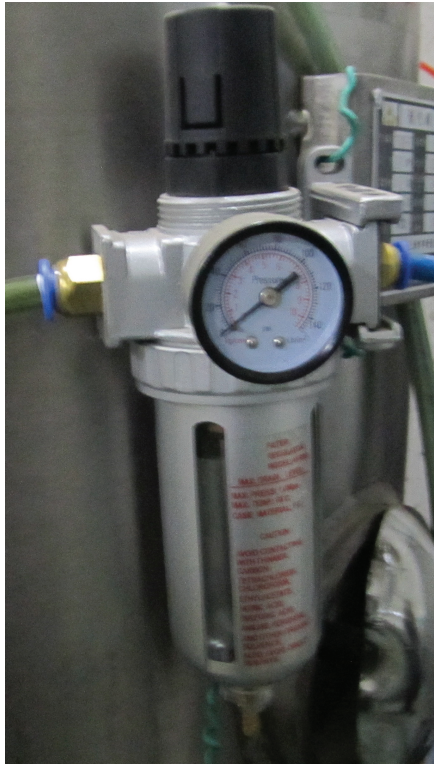
Figure 7. Oil and water filtering regulator for spraying air brush.
