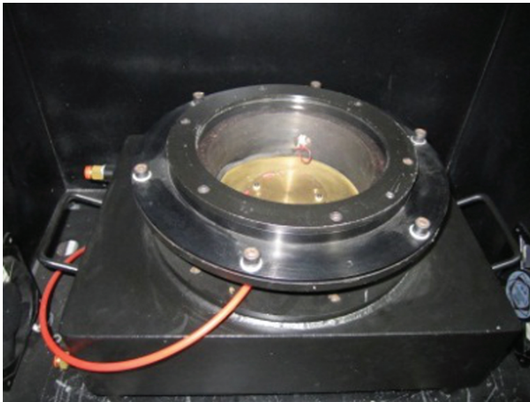
Figure 10. Photo of pressure vessel.
