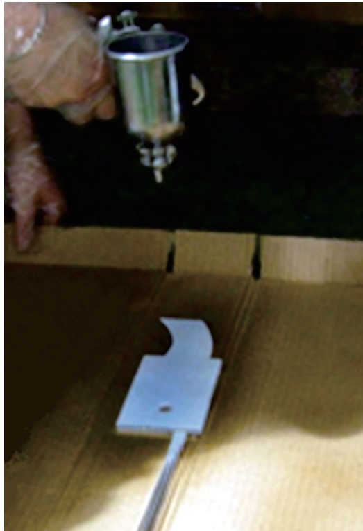
Figure 4. Spraying the paint on the surface.
