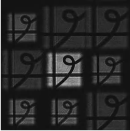
Figure 7.8 Amplitude reconstructions of the “three wires” hologram using four numerical gratings in the algorithm.
