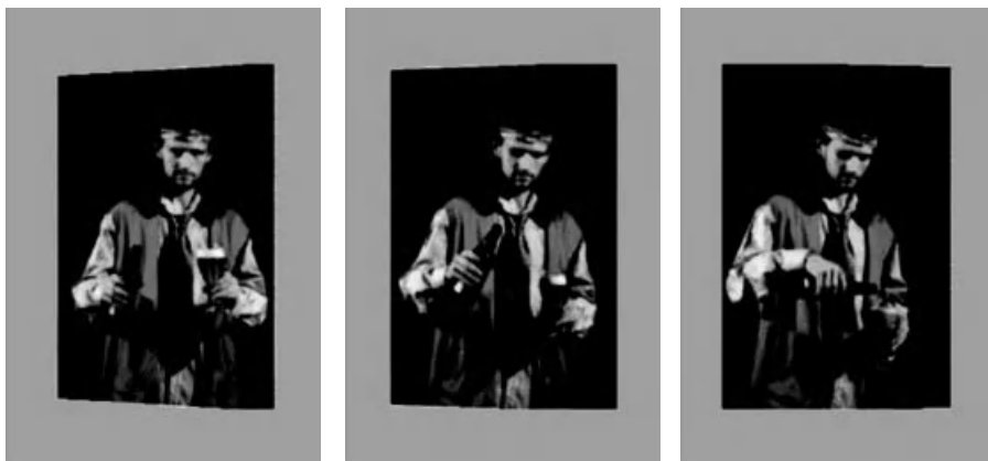
Figure 4.7 Three frames of the reconstructed 3D moving object from i-Lumogram; the total number of views is 640. (Source: With kind permission of Geola UAB, Vilnius, Lithuania.) (Please find a color version of this figure on the color plates.)
