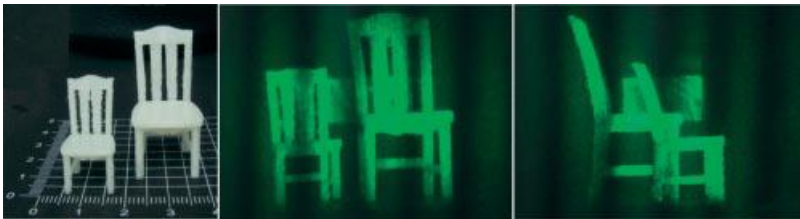
Figure 3.25 Printed model of chairs scene with 3D printer and views of optical reconstruction of digital holograms captured for this model in the system presented in Figure 3.17. (This figure also appears on page 89.)
