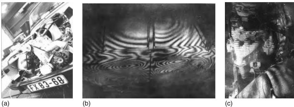
Figure 18.5 Investigation of the automotive parts: (a) the car under investigation, (b) the interferogram of the car body, and (c) the interferogram of the engine block of the car (c).
