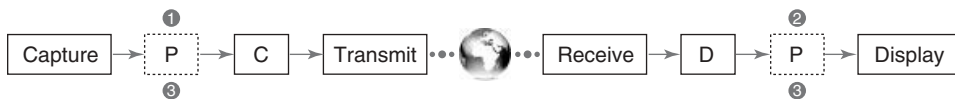
Figure 3.3 The chronological relationship between processing (P), compression (C), and decompression (D), and transmission; options (1), (2), (3) refer to the locations of the processing module.
