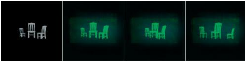
Figure 3.19 3D model of scene composed of chairs and the three views of holographic reconstruction. (This figure also appears on page 82.)
