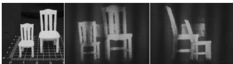
Figure 3.25 Printed model of chairs scene with 3D printer and views of optical reconstruction of digital holograms captured for this model in the system presented in Figure 3.17. (Please find a color version of this figure on the color plates.)
