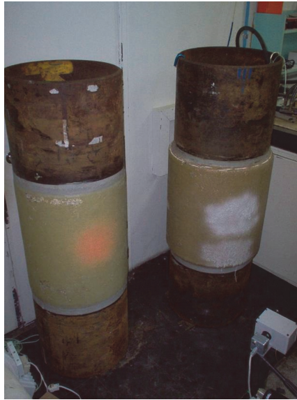
Figure 7.13 Pipe samples with composite repairs (reprinted from Willemann et al. 36 with permission).
