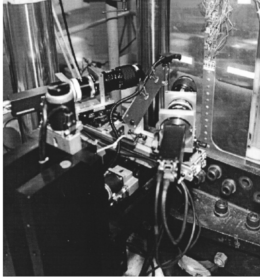
Figure 8.9 Stereovision system for local image acquisition (reprinted from Helm et al. 37 with permission).
