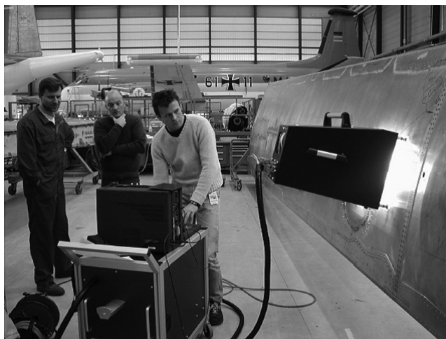
Figure 7.19 Wing inspection using the mobile shearographic system (reprinted from Kalms 42 with permission).
