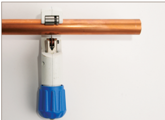
Figure 11.6. Cutting the tube square
