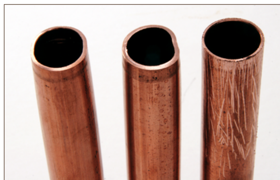
Figure 10.1. Inspect tube for imperfections
