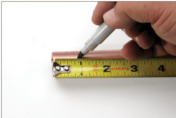
Figure 11.12. Measuring depth of insertion
