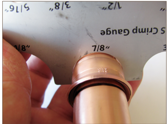
Figure 11.23. Correctly crimped fitting
