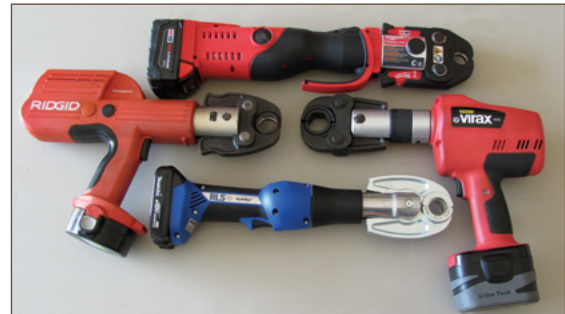
Figure 11.2. Press tools and jaws
