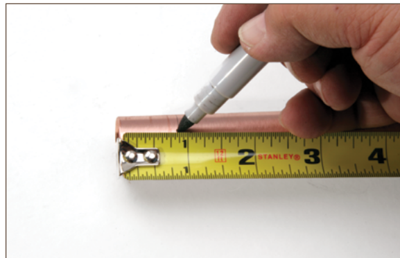
Figure 12.10. Making insertion depth
