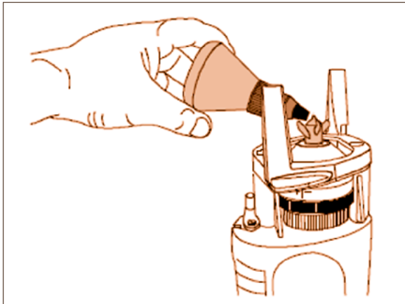
Figure 13.3: Lubricating the drill head
