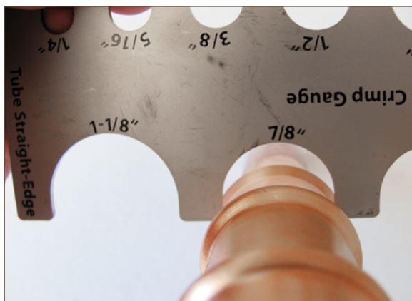
Figure 11.22. Un-crimped or improperly crimped fitting
