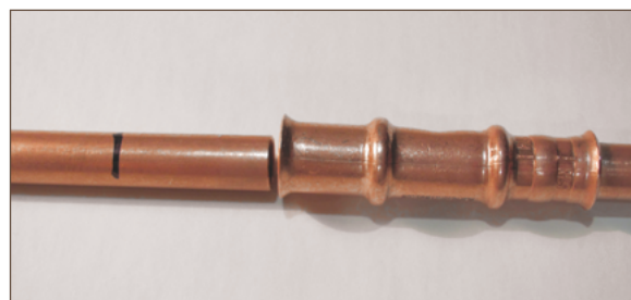
Figure 11.18. Tube marked for insertion into HVACR fitting
