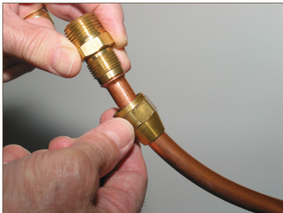
Figure 9.1. Flare Fitting/Flared Joint During Assembly
