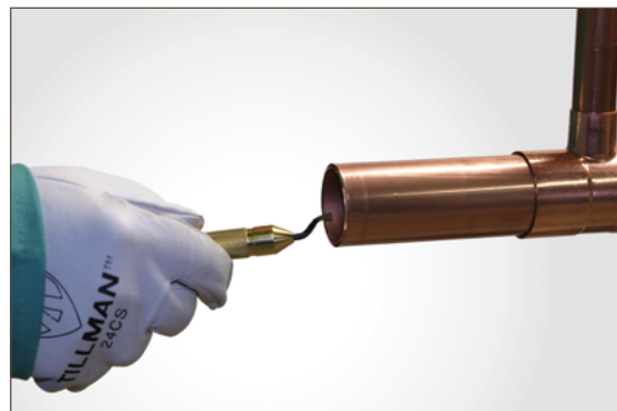
Figure 7.5. Reaming: Deburring Tool
