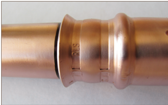
Figure 11.20. Press jaw crimp mark
