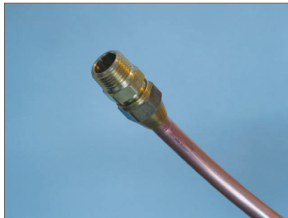
Figure 9.2. Completed Flared Joint
