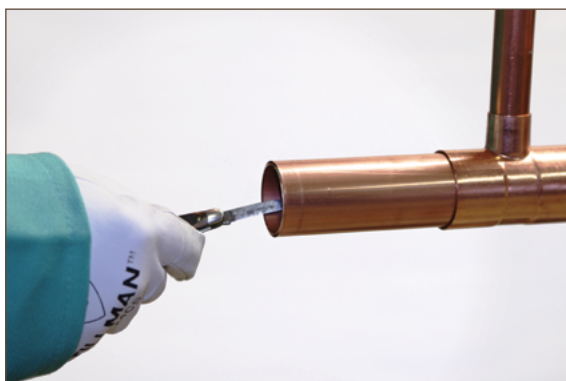
Figure 7.4. Reaming: Pocket Knife
