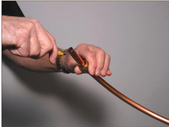
Figure 9.3. Reaming Prior to Flaring the Tube End
