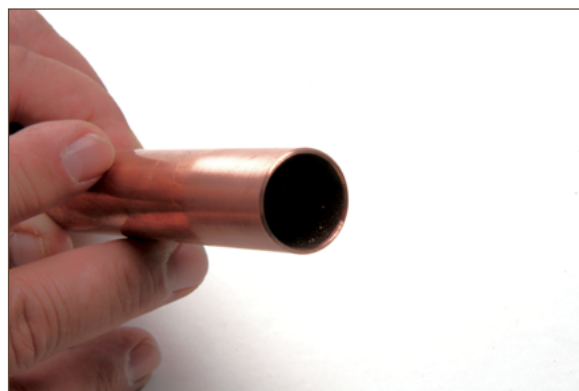
Figure 13.8. Reamed and deburred branch tube end
