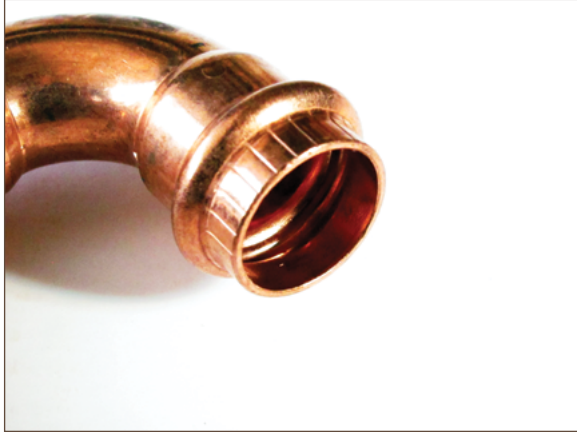
Figure 11.11. Press fitting (NOTE: Missing o-ring)
