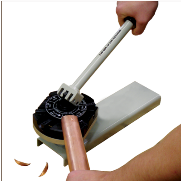
Figure 13.9. Using the notching and dimpling tool
