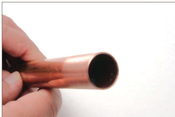
Figure 11.10. Properly prepare tube end
