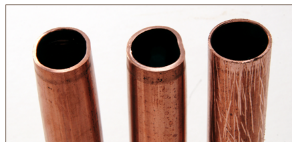
Figure 11.4. Inspect tube for imperfections
