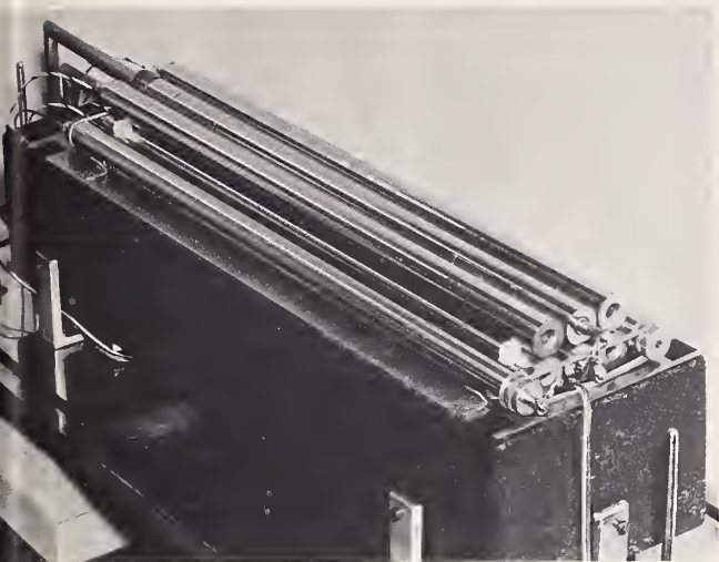
Figure 2. Calculable Cross Capacitor assembled from gage rods.
