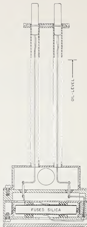
FIGURE 1. Cross section of the capacitance standard.
