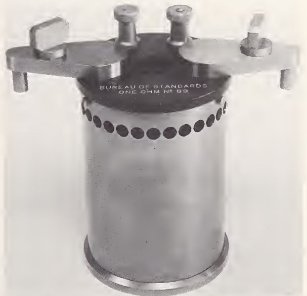
FIGURE 4. Double-walled standard resistor.
