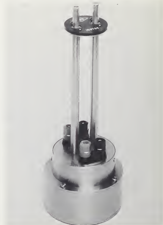
FIGURE 6. Completed capacitance standard.
