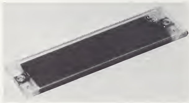
FIGURE 7. Double-wound card resistor cast in epoxy.
