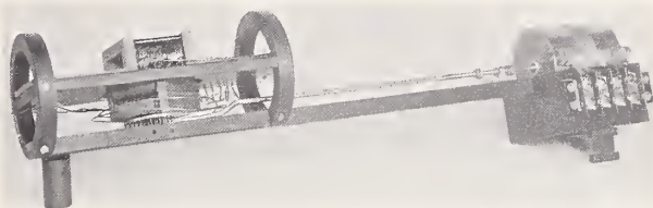
FIGURE 8. Test coil assembly for MH permeameter.
