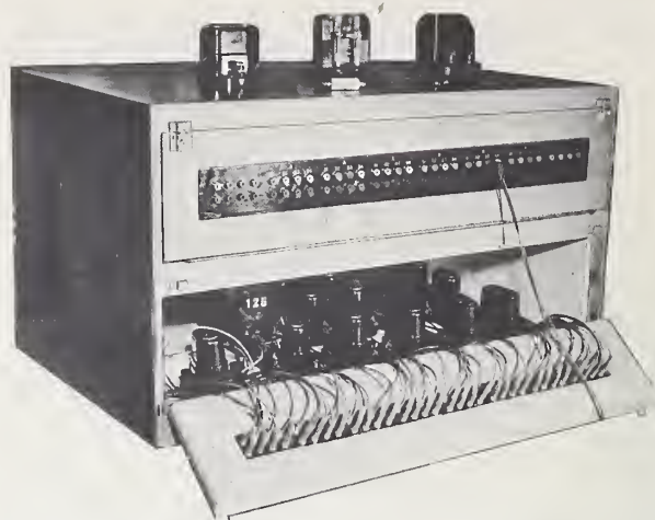
FIGURE 19. Temperature-lagged box used at the National Bureau of Standards in the testing of unsaturated standard cells.
