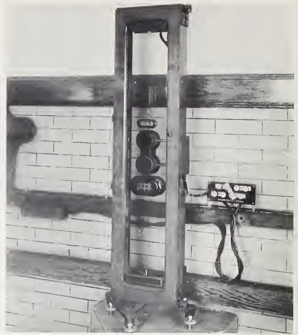
Fig. 1—NBS electrodynamic ac-dc transfer instrument (external multiplier and scale not shown).
