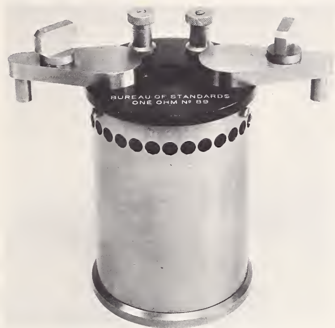
FIGURE 1.— Double-walled standard resistor.
