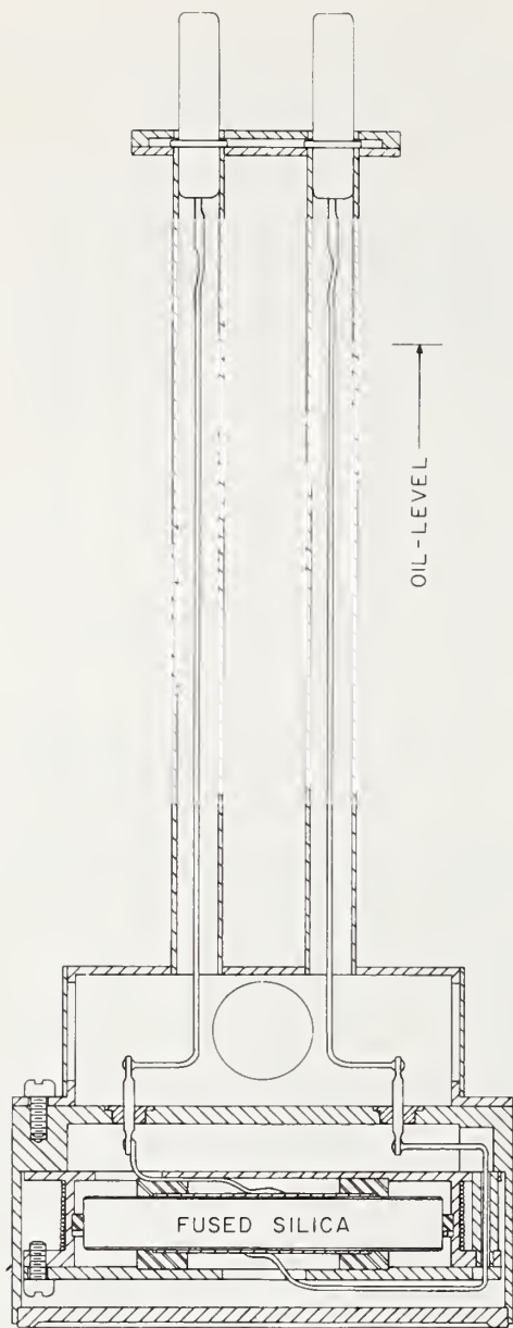
Figure 4. Cross-section of stable 10 pF capacitance standard with fused silica dielectric.
