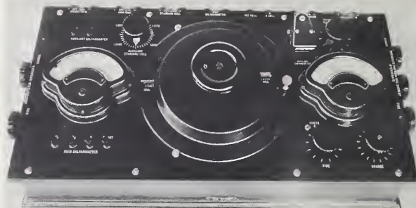
FIGURE 4. Photograph of a Brooks comparator (top view).
